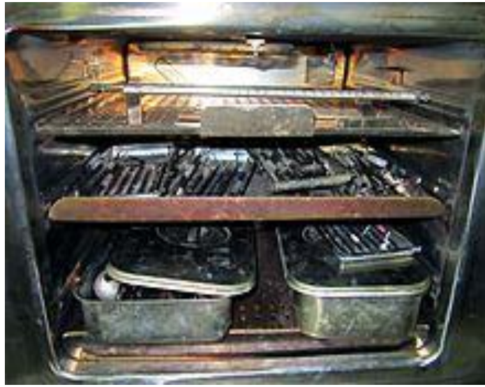
Fig 12.4 Other Autoclave with dental equipment in an autoclave to be sterilized for 2 hours at 150 to 180 degrees Celsius
