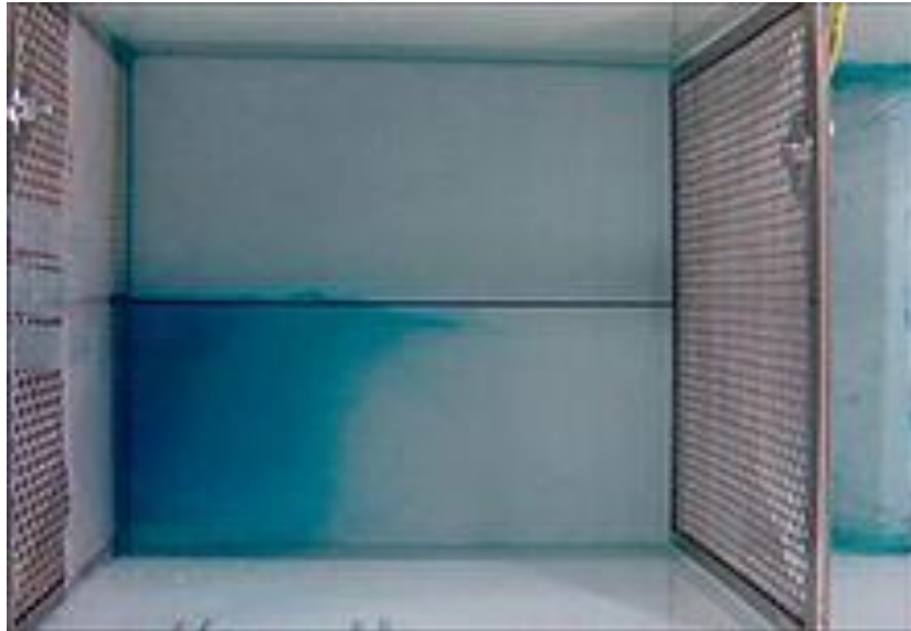
Fig 12.1 Experimental chamber for studying chemo taxis in response to laminar flow
