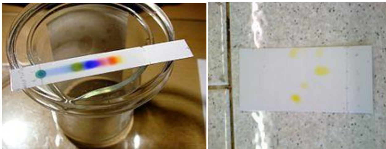
Fig.12.22 Separation of black ink on a TLC plate
