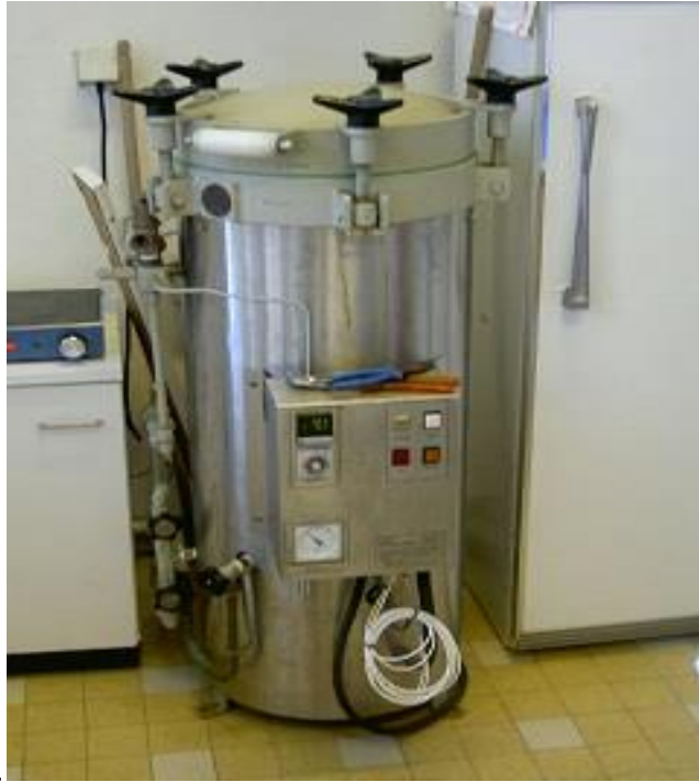
Fig 12.3 This is an autoclave that is used in the medical facility
