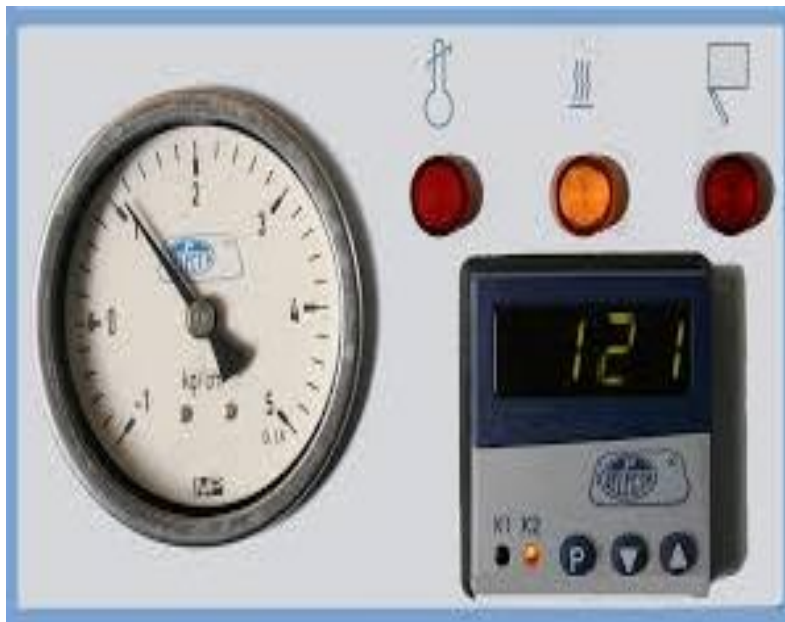
Fig 12.7 The Autoclave must reach 121 degrees Celsius
