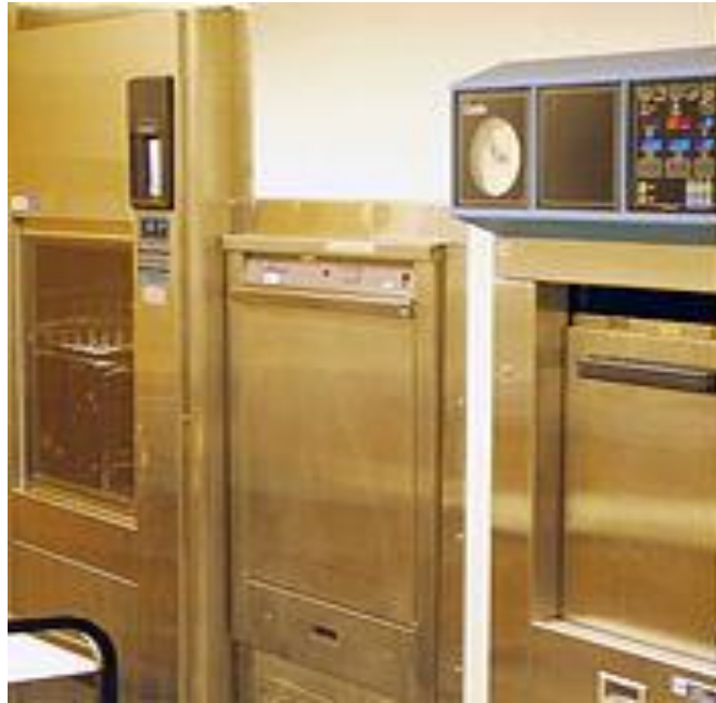
Fig 12.6 The machine on the right is an autoclave used for processing substantial quantities of laboratory equipment prior to reuse, and infectious material prior to disposal. (The machines on the left and in the middle are washing machines.)
