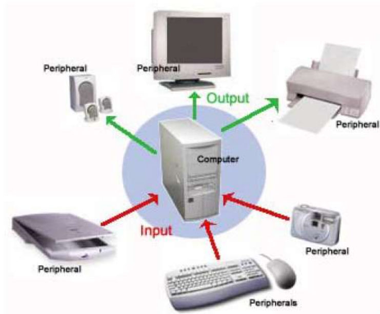
Figure 18: General Purpose Computer System
