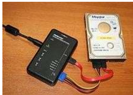
Figure 56: A portable Tableau write blocker attached to a Hard Drive 79
