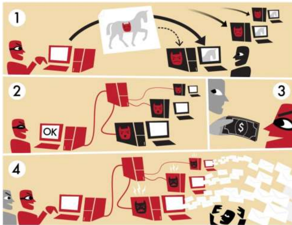
Figure 19: Working of a Trojan horse
