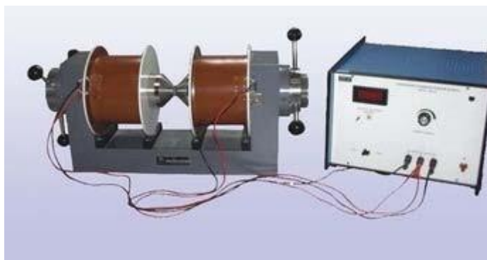
Fig 4.2. Apparatus for the Measurement of Susceptibility of Paramagnetic Solution by Quinck's tube Method
