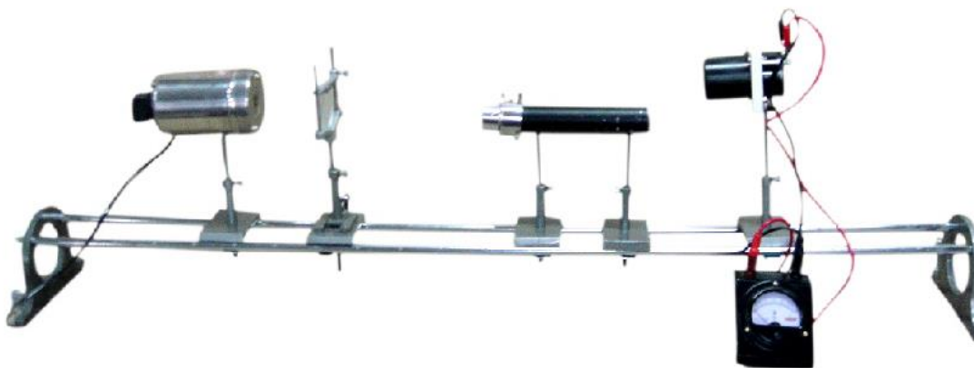
Figure 1: Experimental Setup for studying Malus Law
