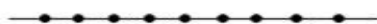
(c) Plane polarized light with electric field vibration perpendicular to plane of paper
