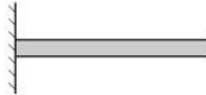
Figure 33: Uniform cylindrical rod fixed at left end.
