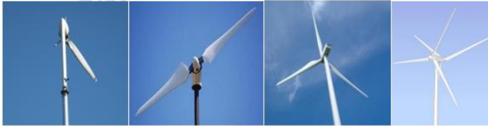
Fig. 9: Single blade, two blade, three blade and multi blade HAWT.
