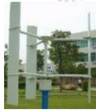
(b) Giromill Wind turbine
