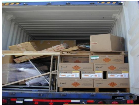
Figure 17.5 Risk of damage (Missing interlayer dunnage)
