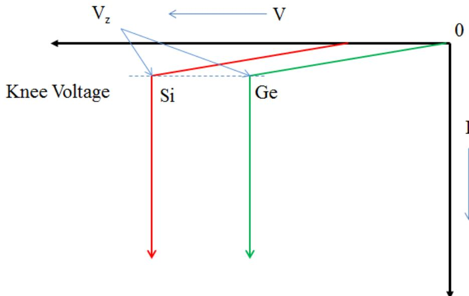
Figure 1. Reverse current in zener diodes made through Si and Ge material
