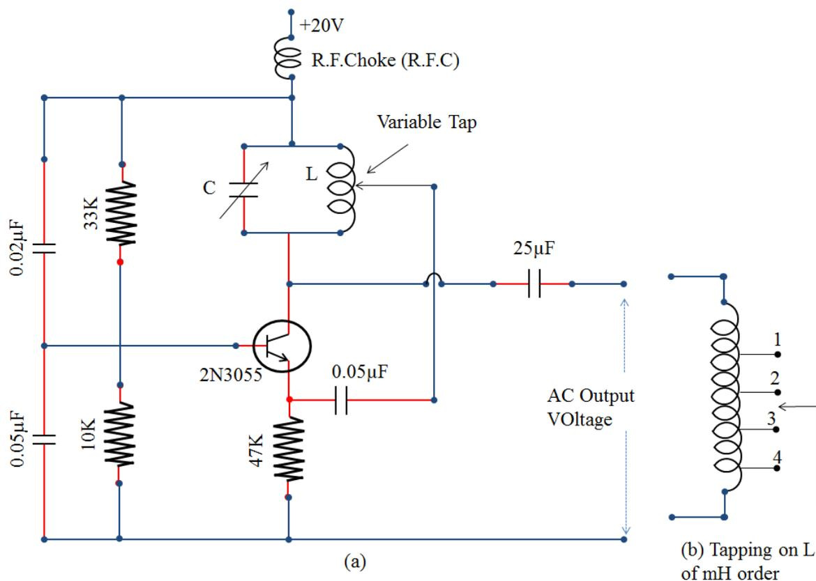
Figure 1. Circuit diagram of Hartley oscillator
