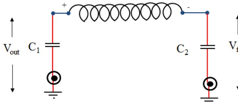
Figure 2: Equivalent Feedback Circuit diagram of Colpitt's Oscillator
