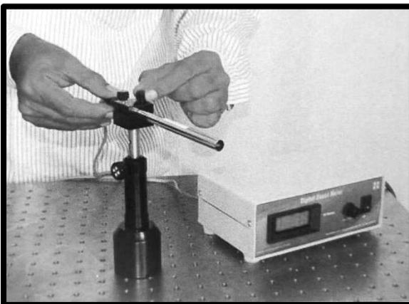
Setting up the Hall Probe with gauss meter.
