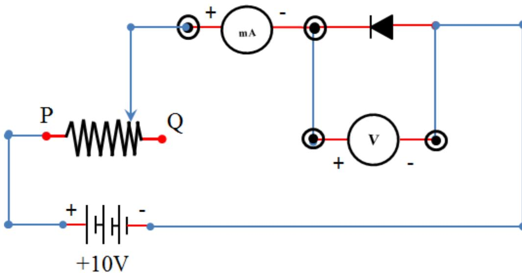
Figure 4. Circuit diagram of reverse bias  $p-n$  junction diode
