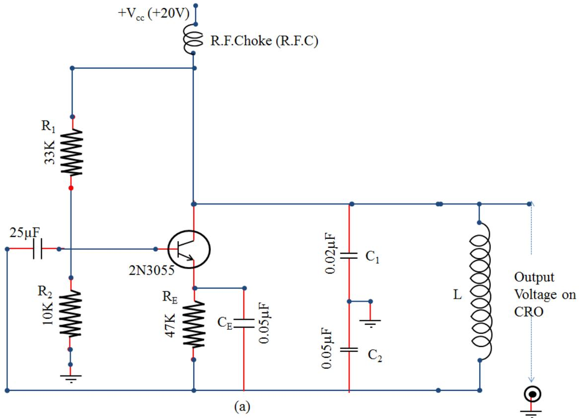
Figure 1. Circuit Diagram of Colpitt's Oscillator
