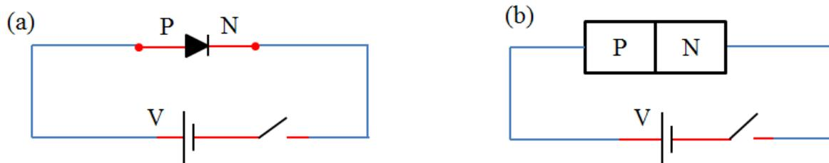
Figure 1. (a) Symbolic representation of a forward bias *pn* junction diode (b) A representation of *p* type and *n* type wafers sandwiched together in a forward bias mode.
