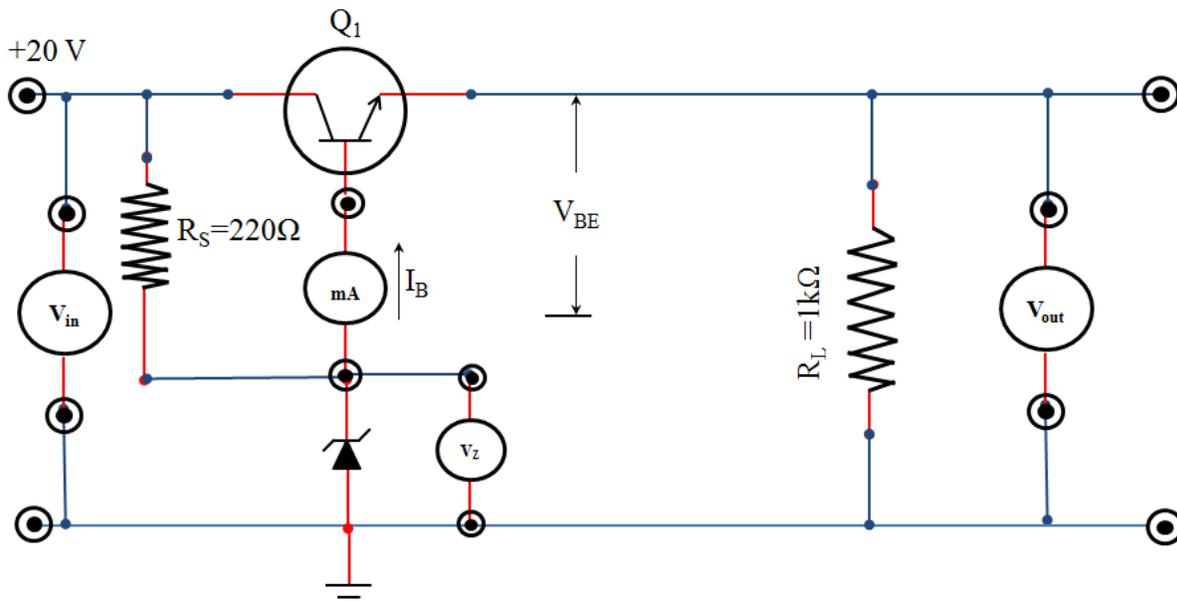
Figure 1. Circuit diagram for a transistorized series voltage regulator
