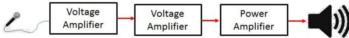
Figure 1. Block diagram of Audio Amplifier showing its various stages
