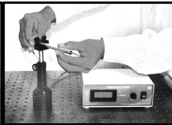
Bring out the Hall Probe with Gauss meter
