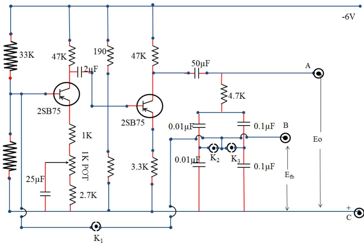
Figure 1: Circuit diagram of a Wien Bridge Oscillator
