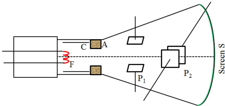
Figure 1. Cathode Ray Tube showing X and Y plates
