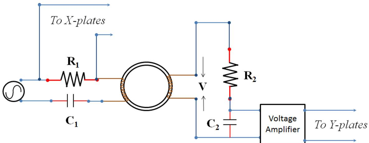
Figure 5. Circuit diagram for tracing the B-H curve
