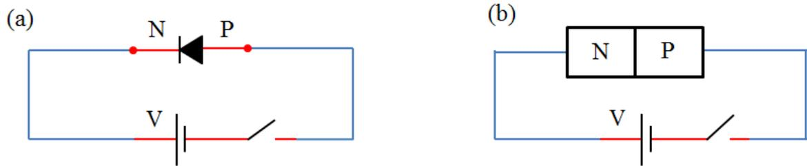
Figure 2. (a) Symbolic representation of a forward bias  $pn$  junction diode (b) A representation of  $p$  type and  $n$  type wafers sandwiched together in a forward bias mode.
