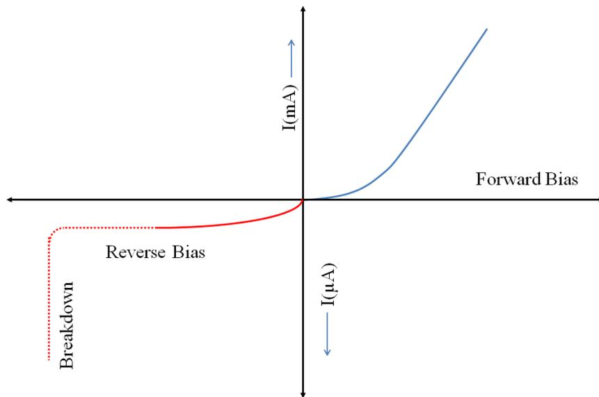
Figure 5. Characteristic curves of forward bias and reverse bias circuit.
