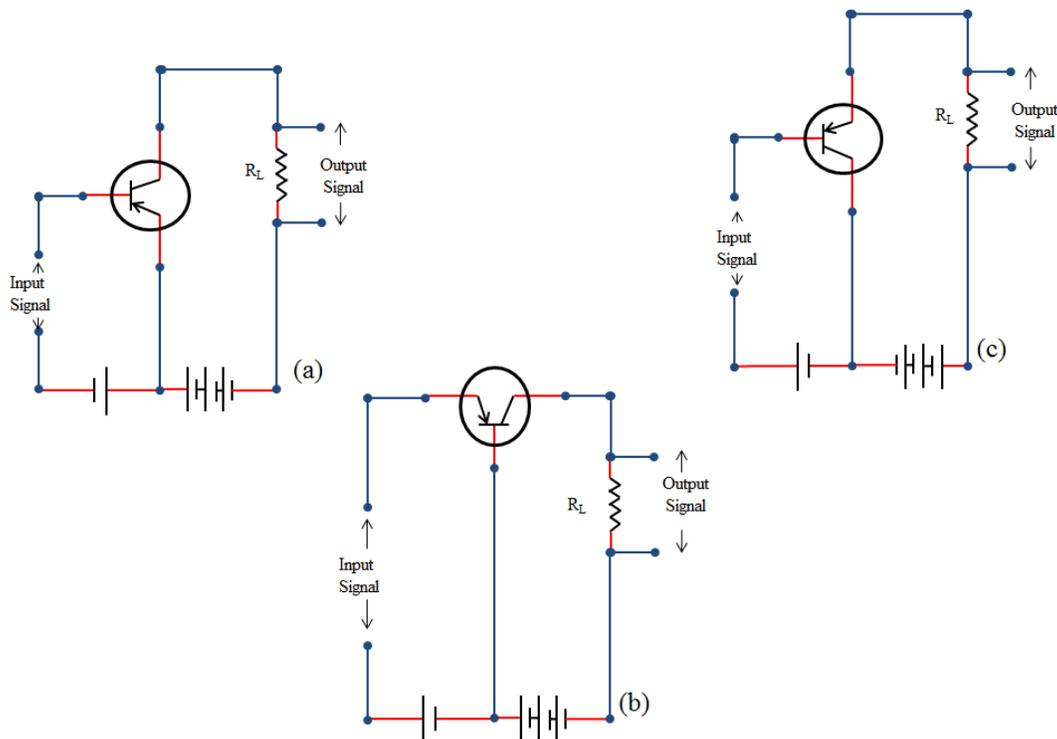
Figure 1(a) Common Emitter (b) Common Base (c) Common Collector circuit diagrams
