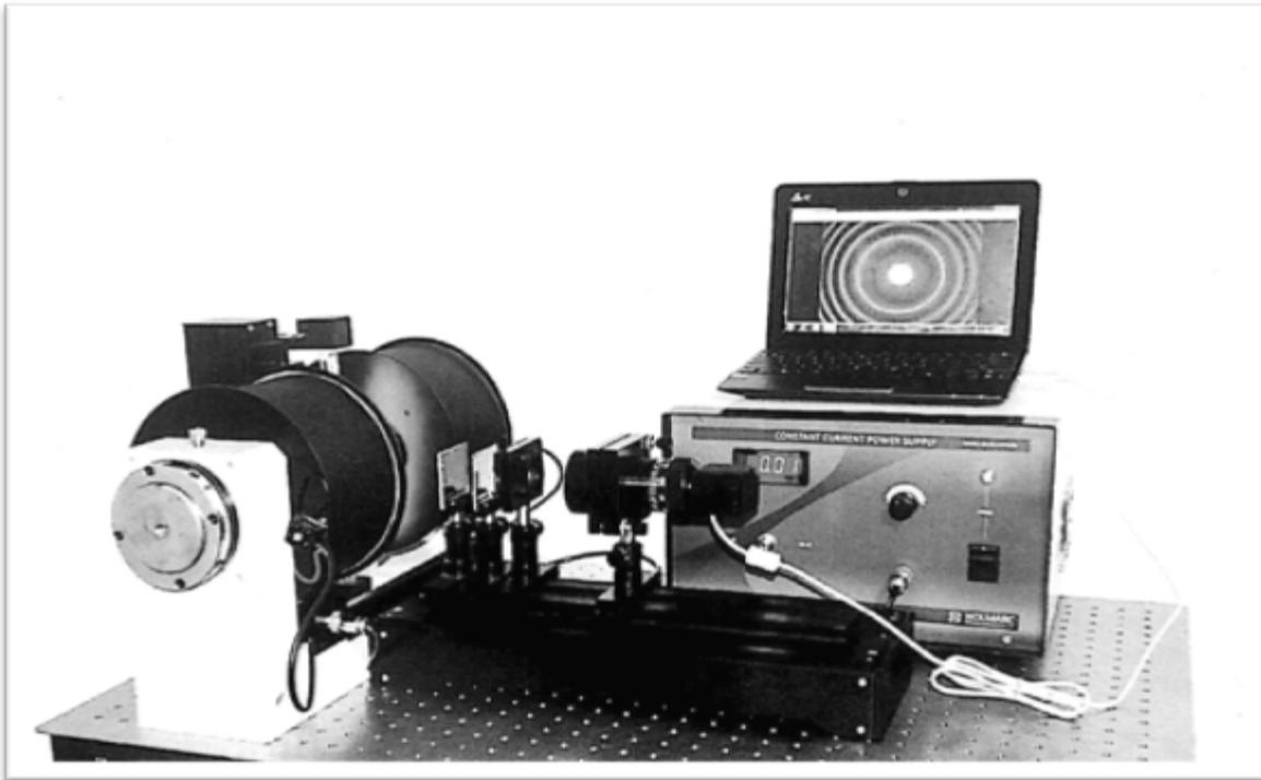
Figure 1: A setup of the Zeeman Effect on a vibration less table
