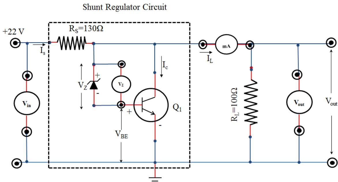
Figure 2. Circuit diagram for a transistorized shunt voltage regulator
