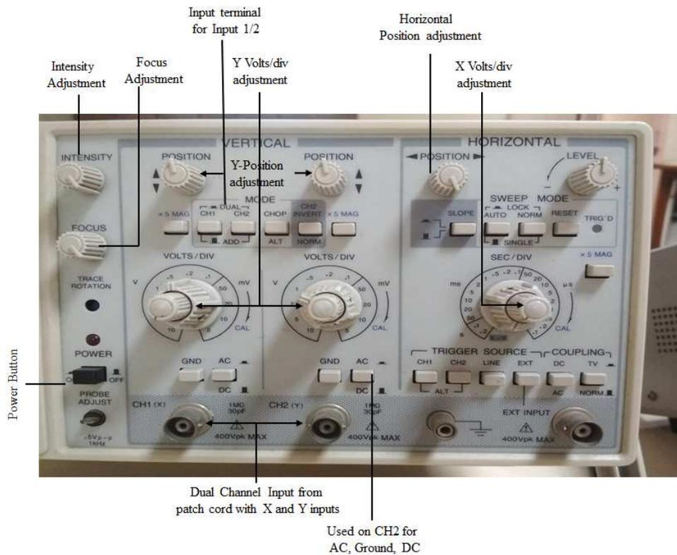
Figure 7. Some useful functions for tracing a curve on CRO
