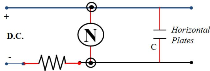
Figure 3. A block diagram showing the basic time-base circuit.
