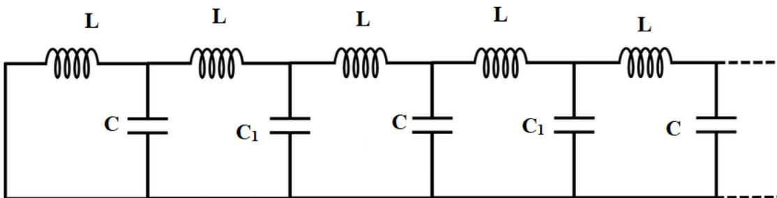
Figure 5: Electrical analog of one dimensional diatomic lattice
