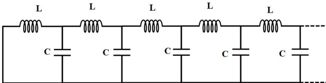
Figure 4: Electrical analog of one dimensional monoatomic lattice
