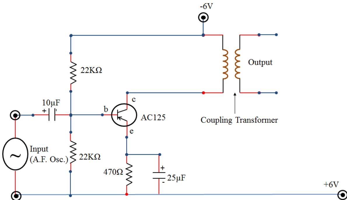
**Figure 1. Circuit diagram of single stage transformer coupled amplifier.**
