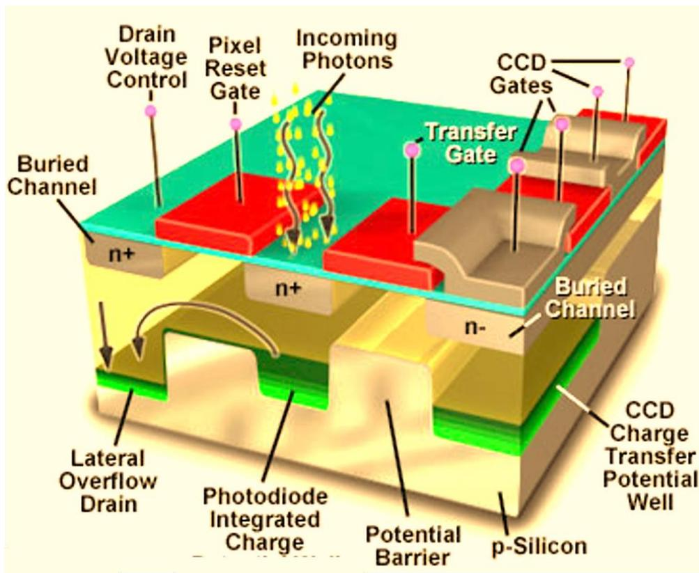
**Figure 7.13 Working of charge coupled device**
