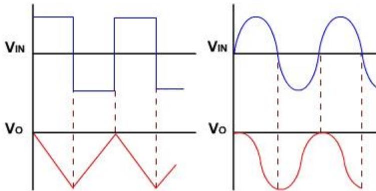
**Fig. 5.22: input and output waveform of an Integrator circuit**
