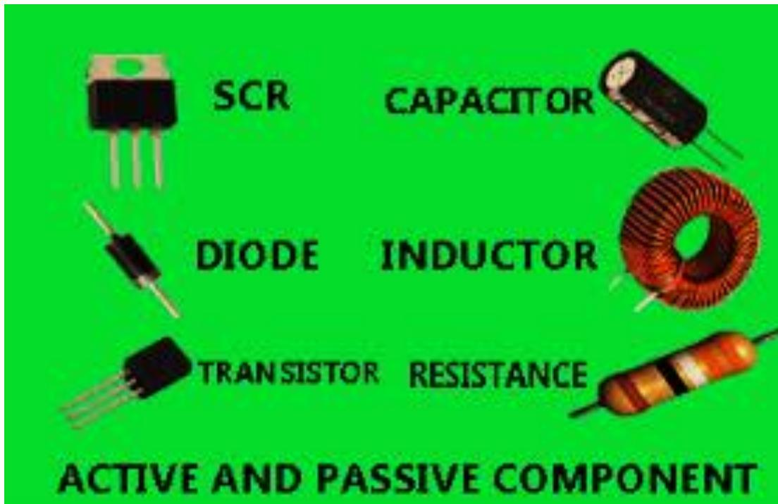
**Figure 7.10** Some of the active and passive components
