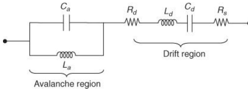
**Figure 1.17** Equivalent circuit of IMPATT diode
