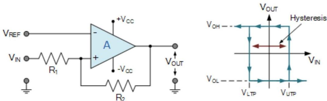
Figure 4.27 Non-inverting Comparator Circuit with Hysteresis
