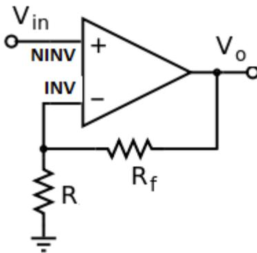
**Fig.5.3: Analog Noninverting amplifier**
