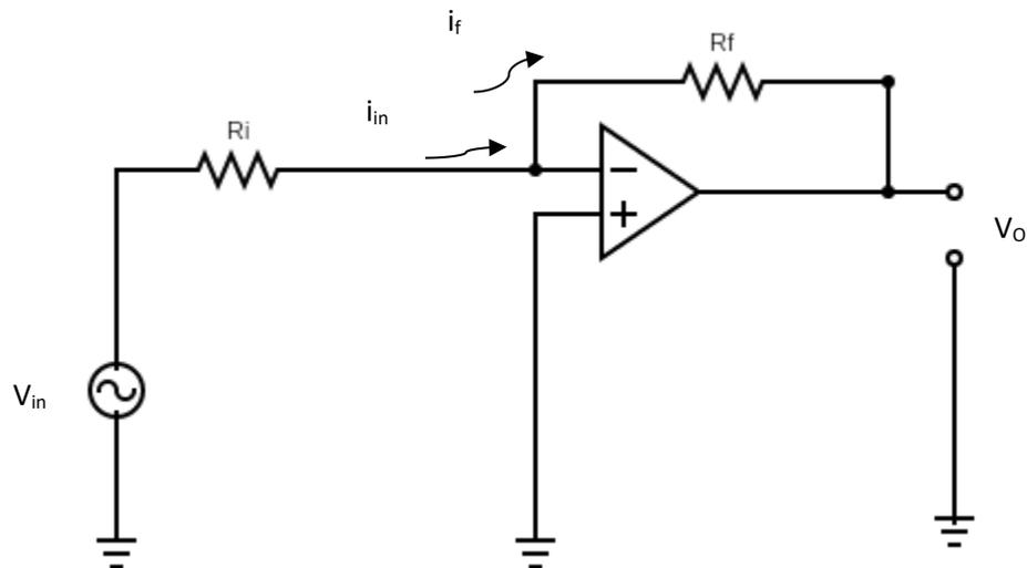
Figure 4.10 Inverting Op-Amp
