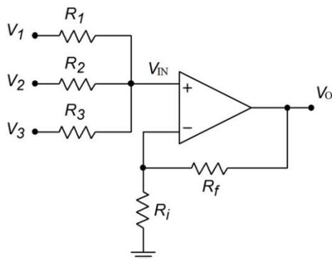
**Fig. 5.6: 3-input Noninverting Voltage Adder Amplifier**
