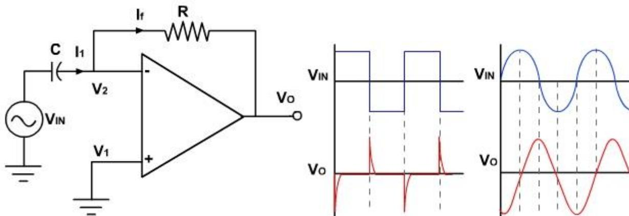
**Fig. 5.19: A differentiator circuit and its output**
