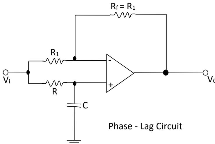
Fig. 6.2 Phase lag circuit
