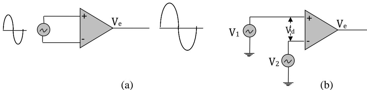
**Figure 4.3 Double-ended (differential) operation.**
