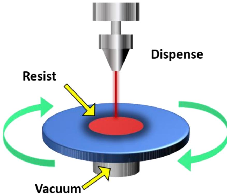
**Figure 7.7**Coating photo resist layer
