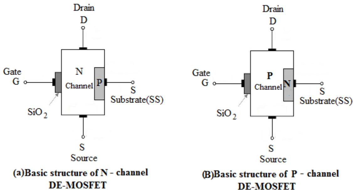
**Figure 3.12 Basic structure of DE-MOSFET**
