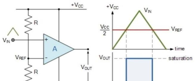
Figure 4.23 Non inverting Comparator Circuit
