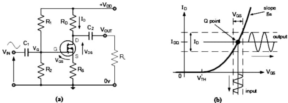
**Figure 3.23 Common source N channel E-MOSFET amplifier**
