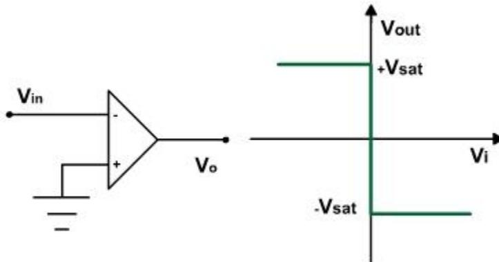
**Fig. 5.9: zero crossing detector**
