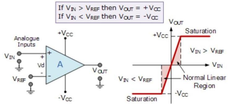
**Figure 4.21 Op-Amp Comparator circuit**
