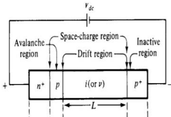
**Figure 1.15 Construction of IMPATT diode**
