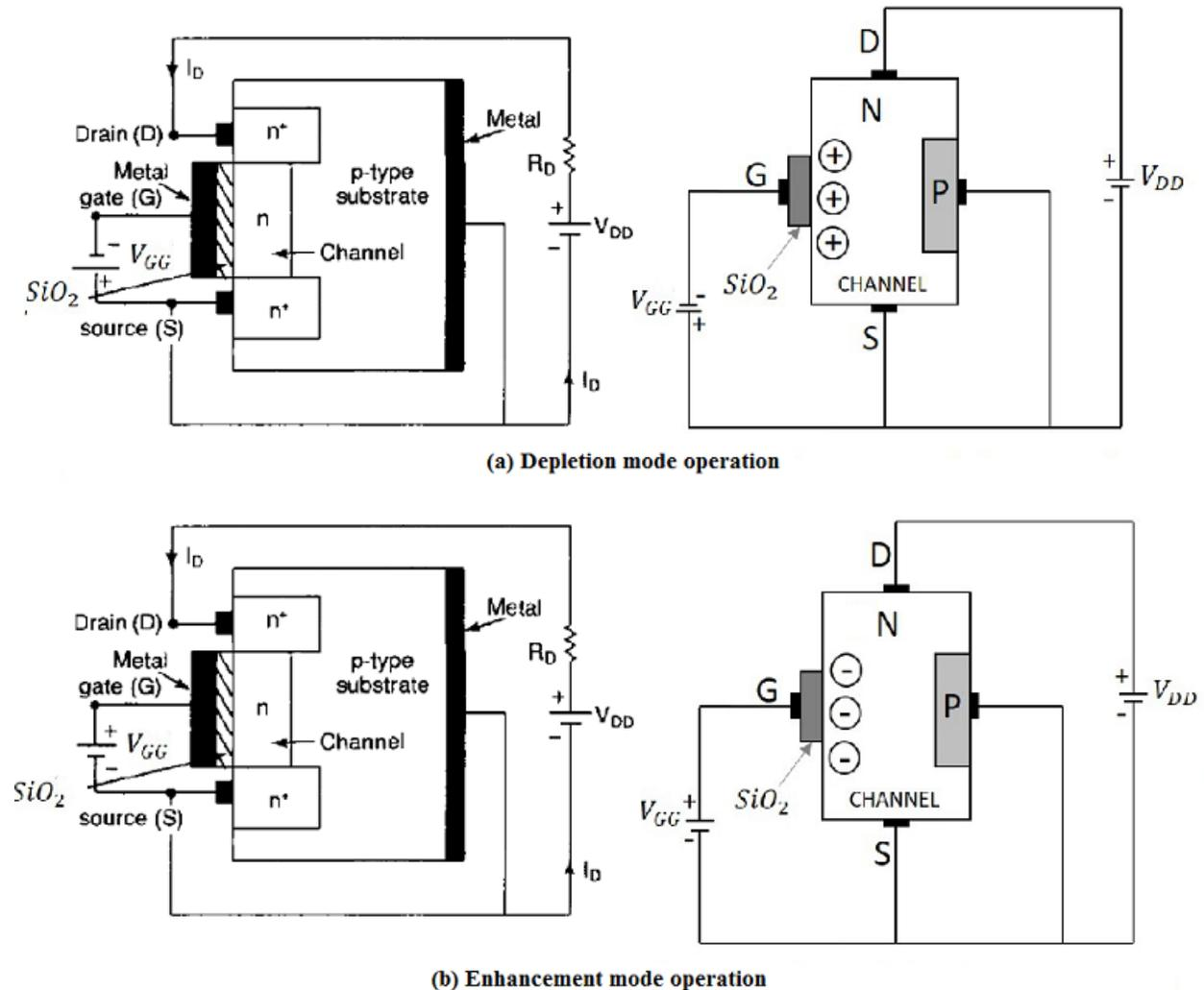
**Figure 3.14 Working of DE-MOSFET**
