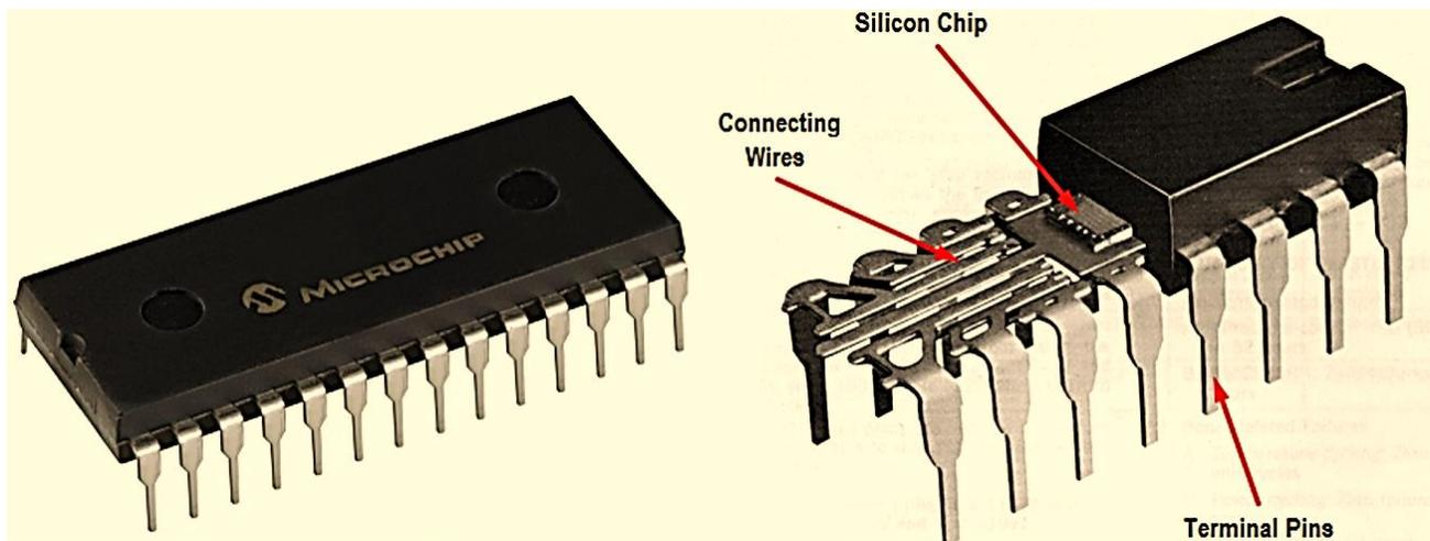
**Figure 7.2 Monolithic IC in plastic package**
