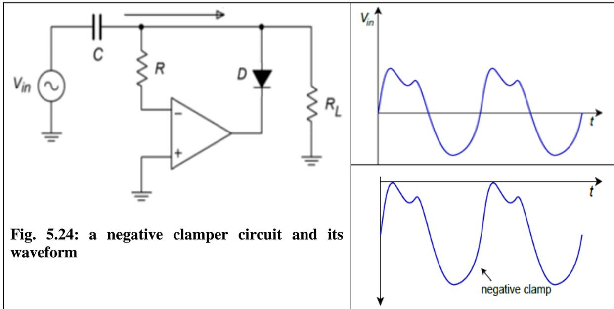
**Fig. 5.24:** a negative clamper circuit and its waveform
