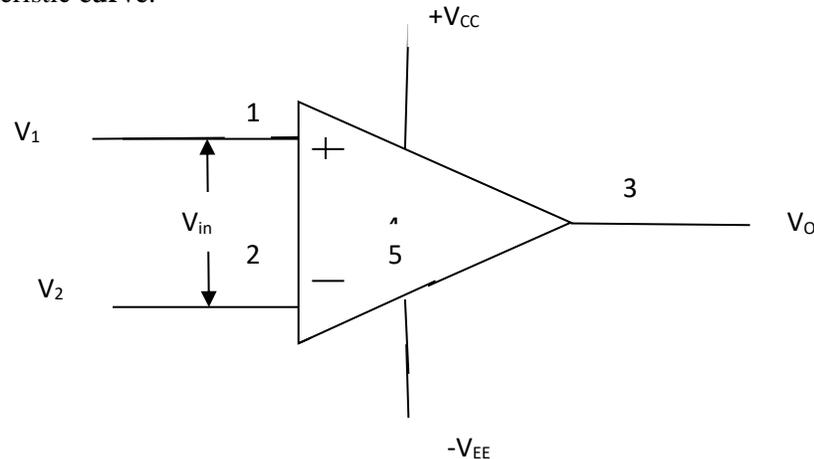
$$V_O = A_v V_{in} = A_v (V_1 - V_2)$$
