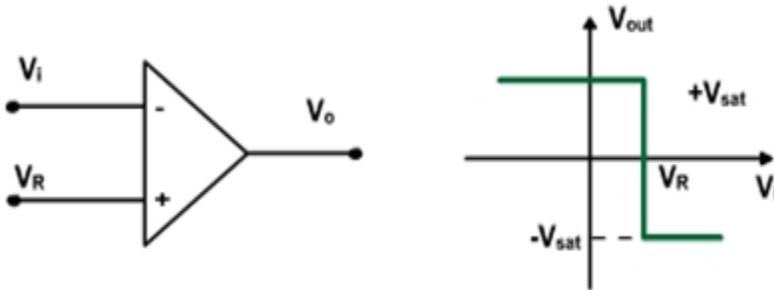
**Fig. 5.7: The basic circuit of a comparator**
