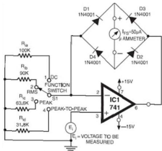
Figure 6.6: Universal High Resistance DC Voltmeter
