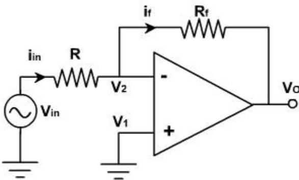
**Fig.5.2: Analog inverting amplifier**
