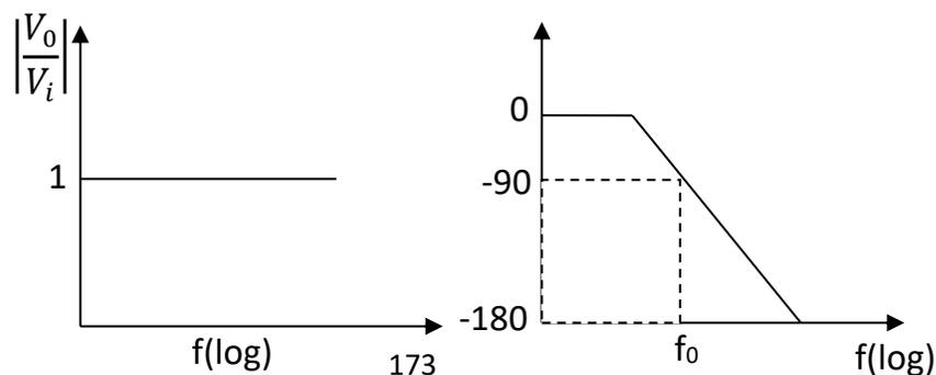
**Fig. 6.3 Bode plot of phase lag circuit**
