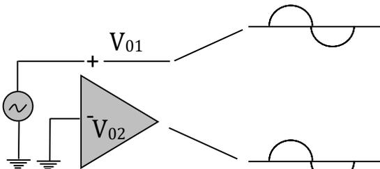
Figure 4.5 Double-ended output with single-ended input
