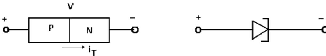
**Figure 1.10** Symbol of tunnel diode
