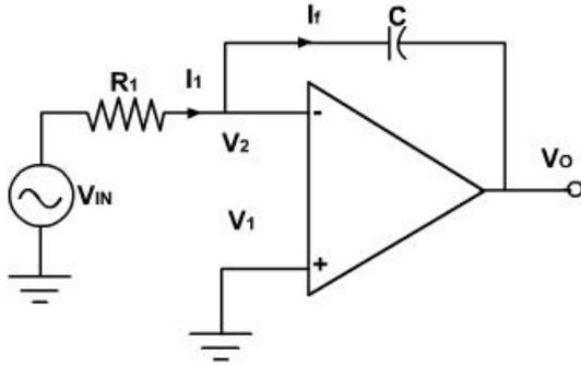
**Fig. 5.21: An Integrator circuit**
