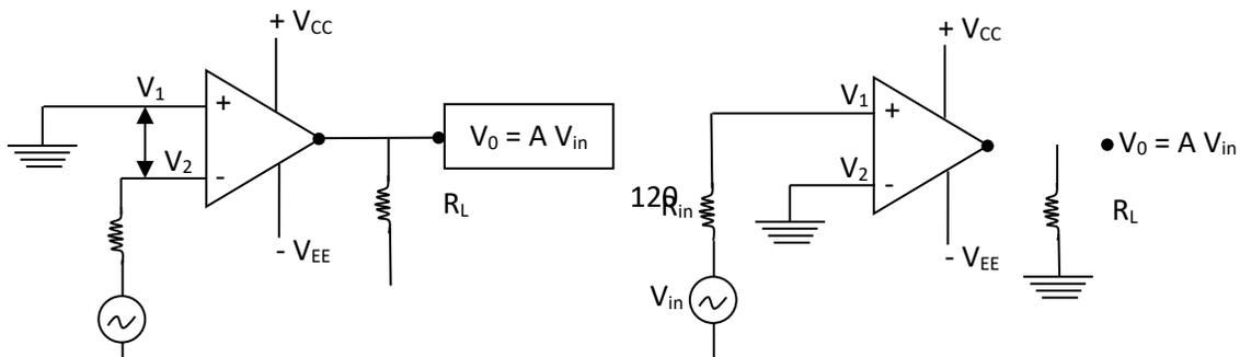
Inverting AmplifierNon-inverting Amplifier4.6 Closed Loop Gain:
