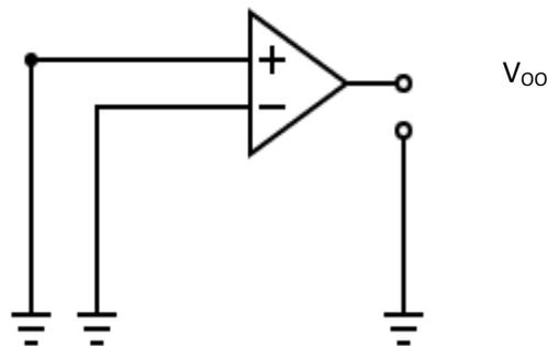
Figure 4.12 Output Offset Voltage
