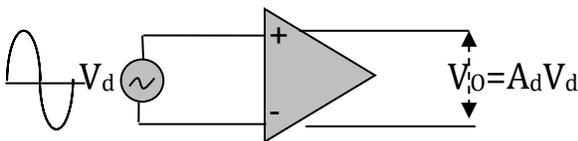
Figure 4.7 Differential-input, differential-output operation.
