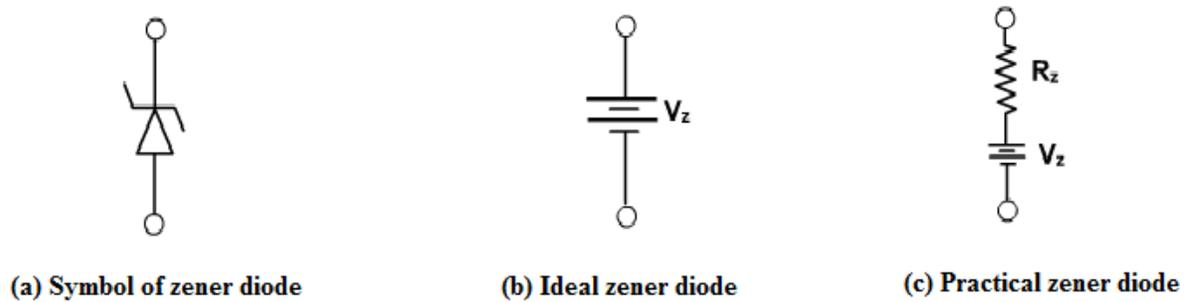
**Figure 1.5 Zener diode: symbol and equivalent circuit**
