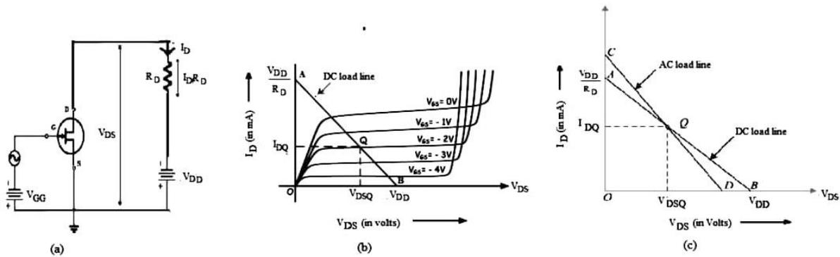
**Figure 3.10 Load line and Operating point(Q point)**
