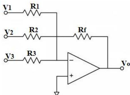
**Fig. 5.5: 3-input Inverting Voltage Adder Amplifier**
