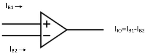
Figure 4.14 Input offset Current
