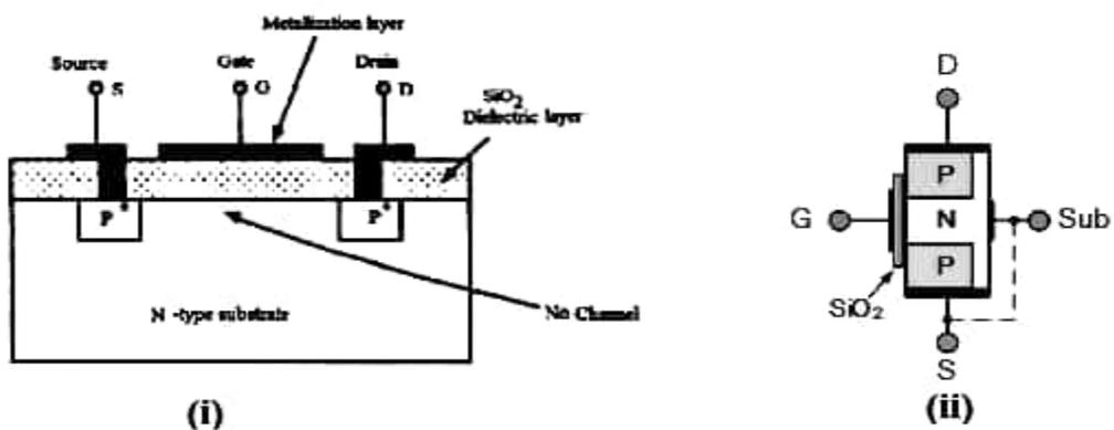
**(b) Basic structure of P-channel MOSFET**
