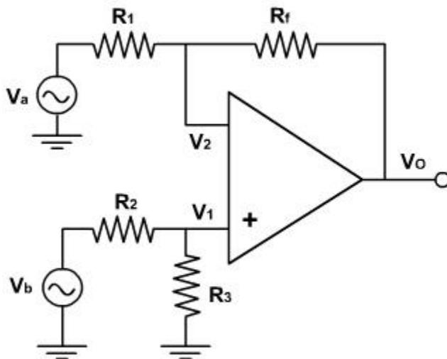
**Fig. 5.4: Basic Differential Amplifier**
