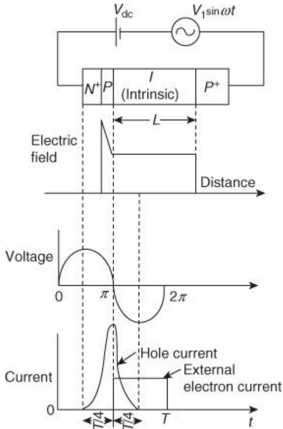
**Figure 1.16** IMPATT diode operation
