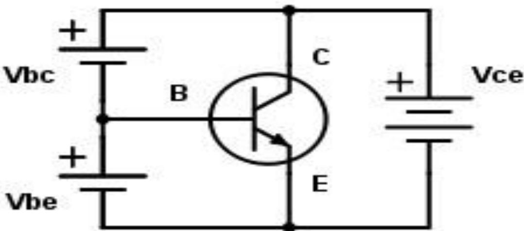
**Figure 4** NPN Bipolar Transistor circuit
