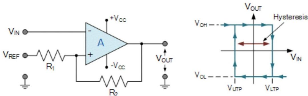
Figure 4.26 Inverting Comparator Circuit with Hysteresis
