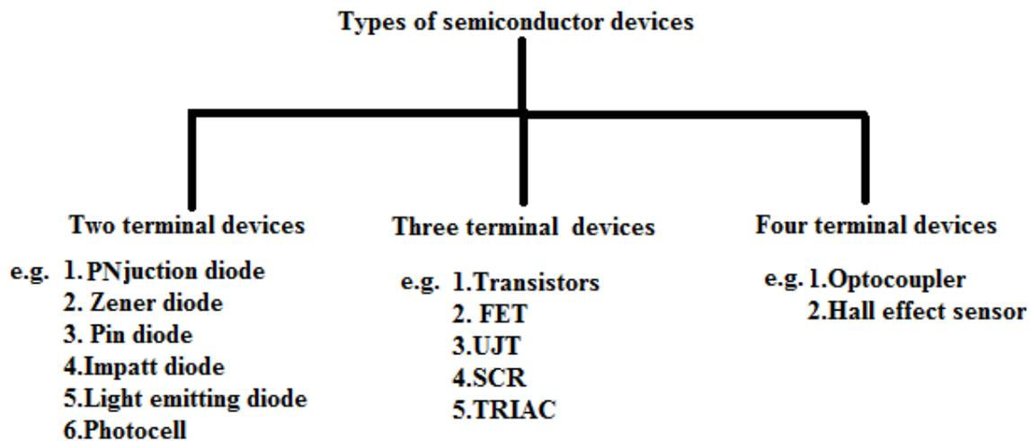
**Figure 1.1 Types of semiconductor devices**
