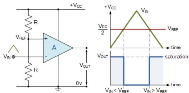
Figure 4.24 Inverting Comparator Circuit
