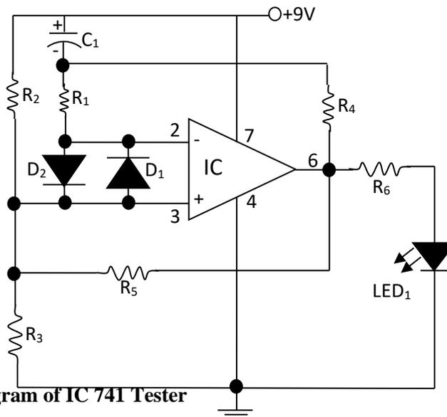
Figure 6.6: Circuit Diagram of IC 741 Tester
