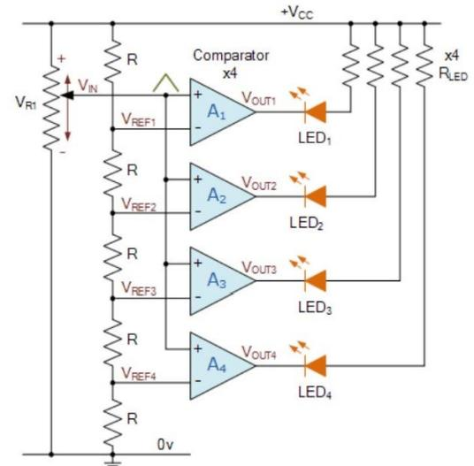
Figure 4.25 Non inverting Comparator Circuit
