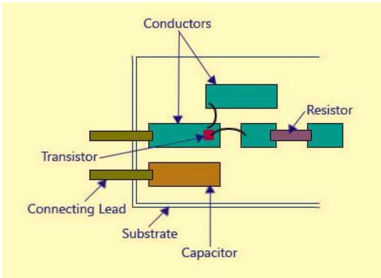
**Figure 7.4 Thick film circuit**
