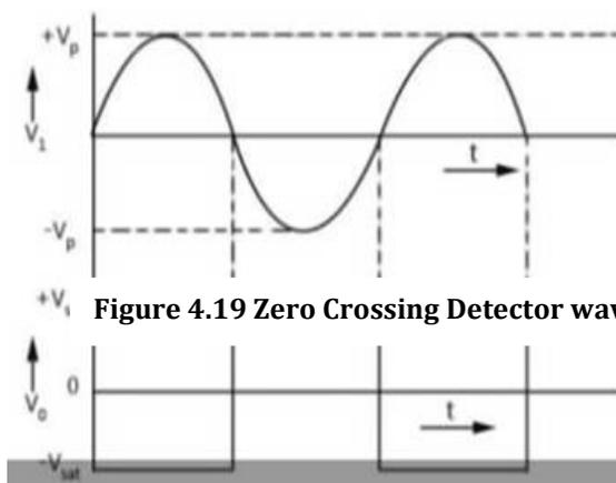
Figure 4.19 Zero Crossing Detector waveform
