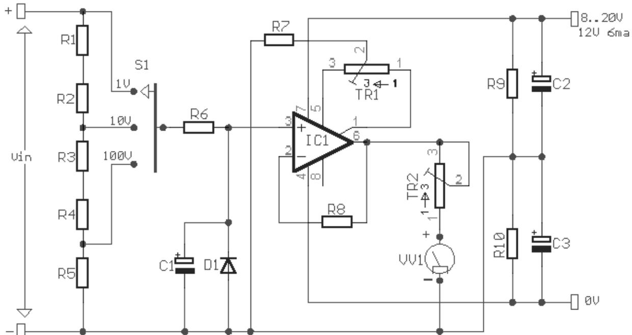
**Figure 6.7: HIGH IMPEDANCE DC-VOLTMETER**
