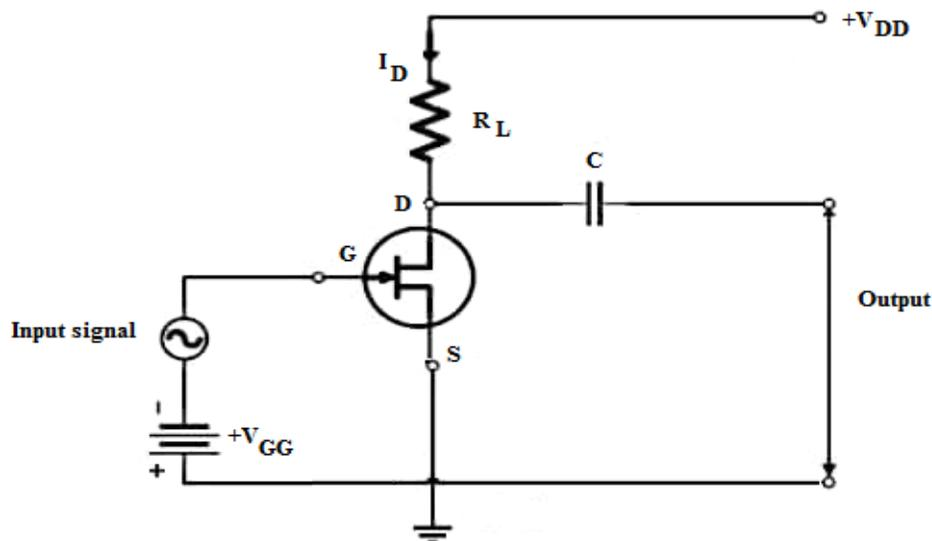
**Figure 3.11 circuit diagram of JFET as an amplifier**
