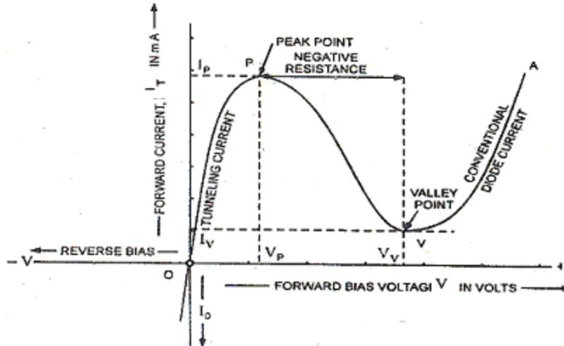
**Figure 1.11 (V-I) characteristics of tunnel diode**
