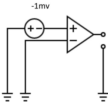
Figure 4.13 input Offset Voltage
