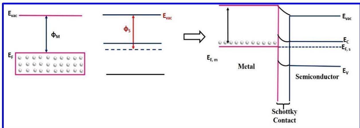
**Figure 7.11 Band structure of metal and semiconductor, when work function of the metal is higher than semiconductor (Schottky contact)**
