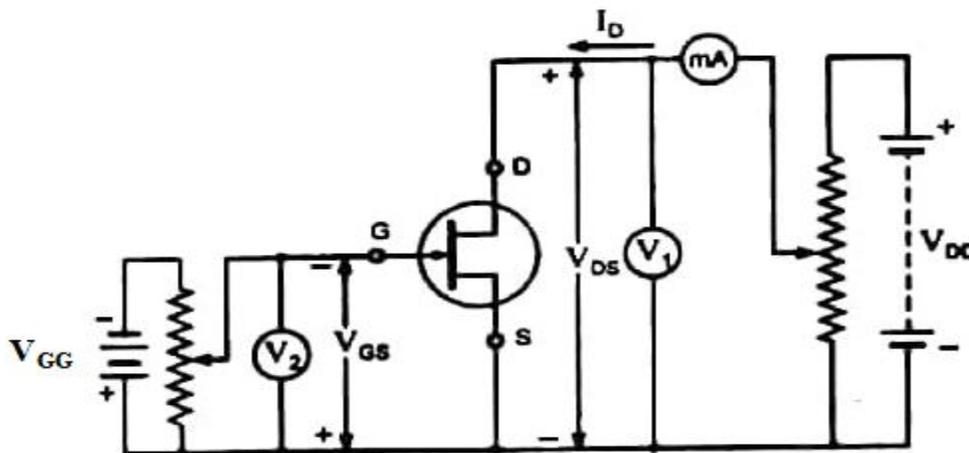
**Figure 3.7** Circuit diagram to study characteristics of JFET
