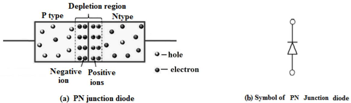
**Figure 1.2 PN junction diode and it's symbol**
