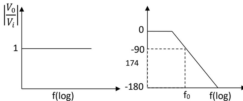
Fig. 6.5 Bode plot of Phase lead circuit
