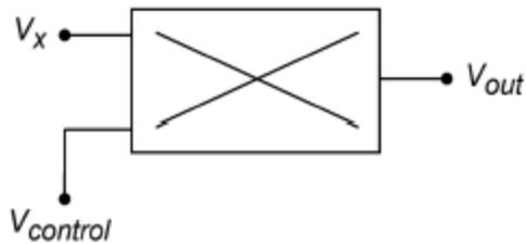
**Fig. 5.17: Multiplication circuit**
