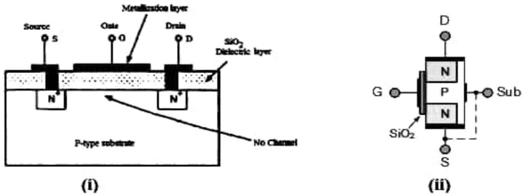
**(a) Basic structure of N-channel MOSFET**
