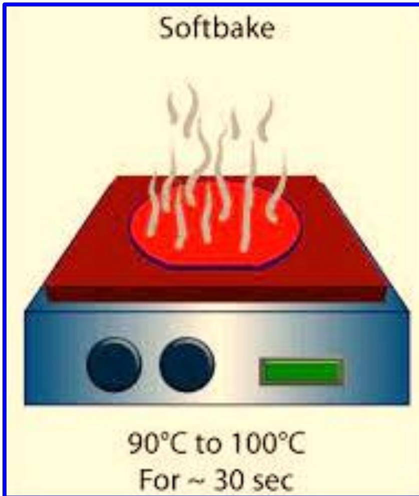
**Figure 7.8 Soft baking step of photolithography**
