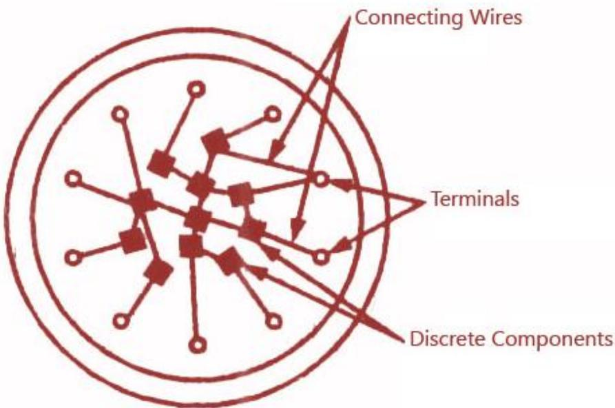
**Figure 7.3 The structure of a hybrid IC**
