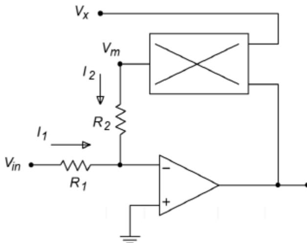
**Figure 5.18: A divider circuit**
