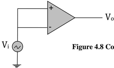
Figure 4.8 Common-mode operation.
