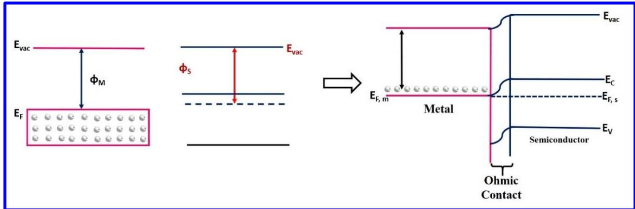
**Figure 7.12** Band structure of metal and semiconductor, when work function of metal is lower than semiconductor (Ohmic contact)
