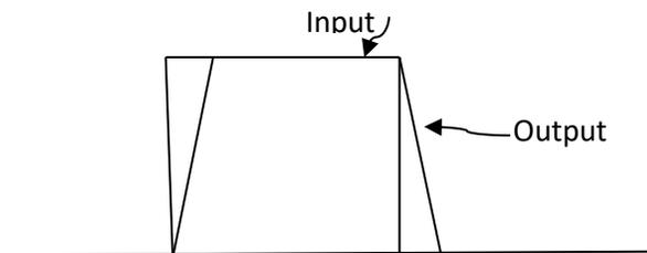
Figure 16 Distortion in signal due to Slew Rate
