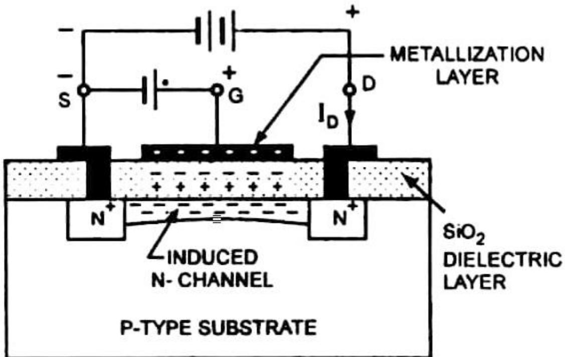
**Figure 3.19 Biasing polarities of N channel E-MOSFET**
