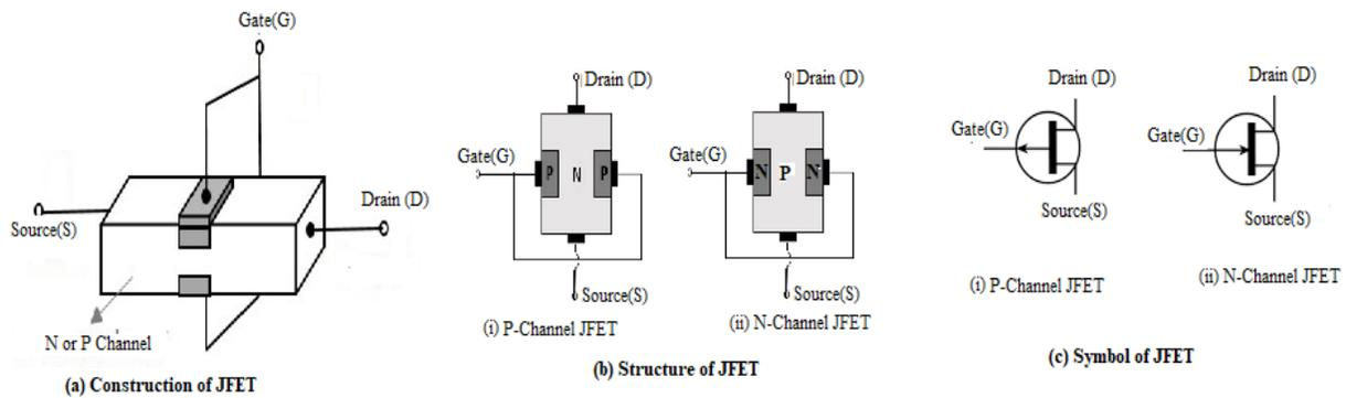
**Figure 3.2 Construction and symbol of JFET**
