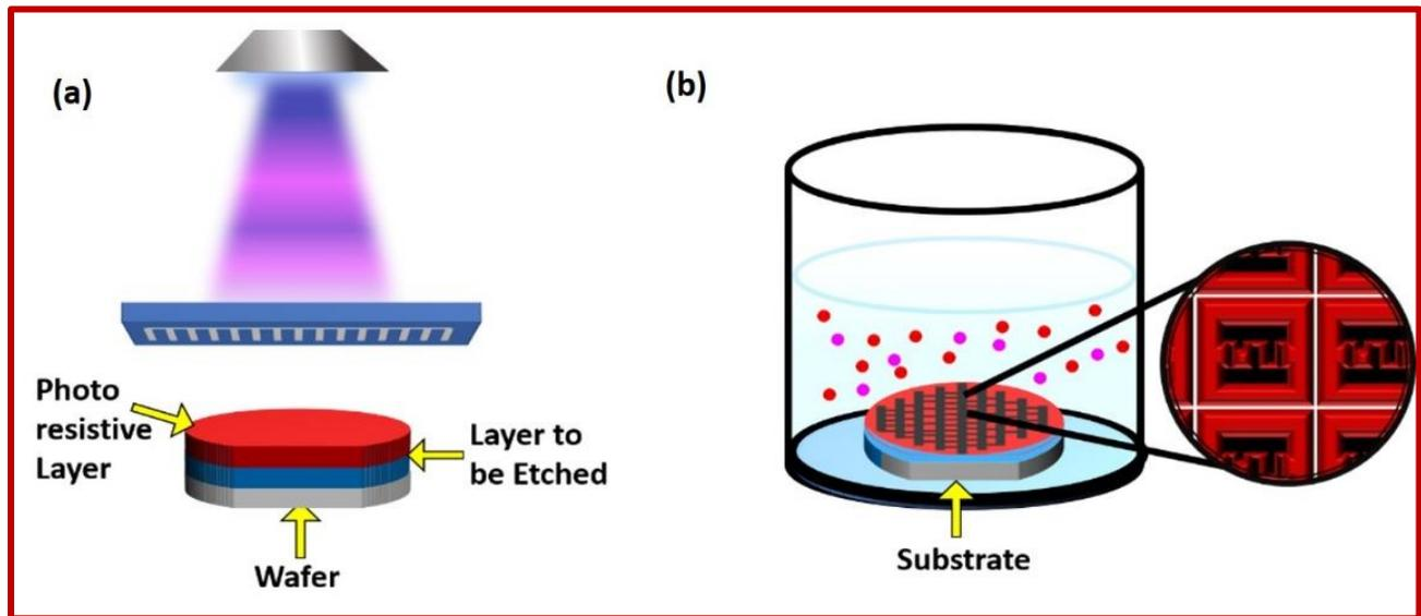
**Figure 7.9 (a) Coating exposure layer (b) Coating developer layer**
