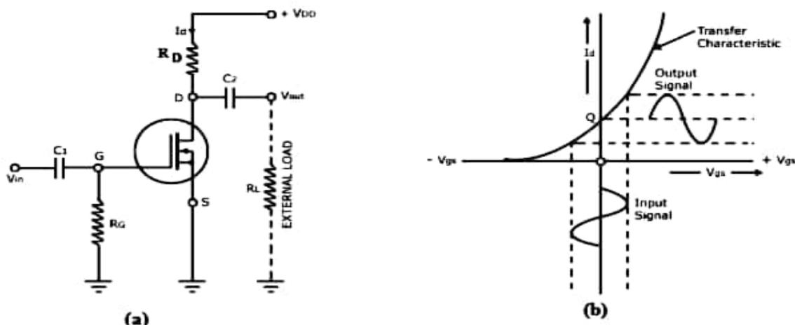
**Figure 3.22 Common source N channel DE-MOSFET amplifier**
