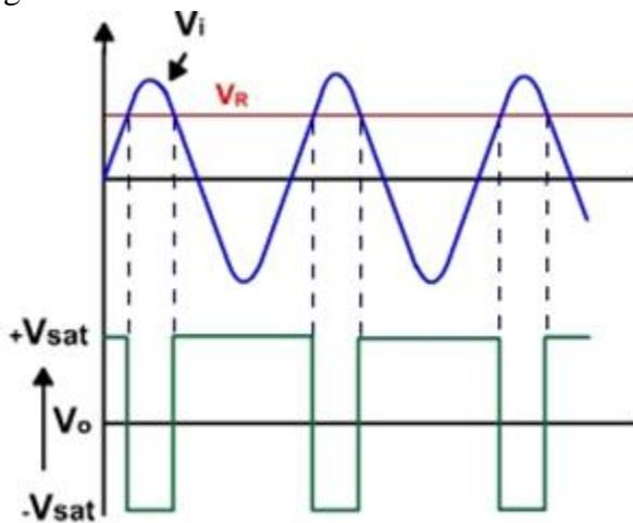
**Fig. 5.8: output of a comparator for a sinusoidal input.**
