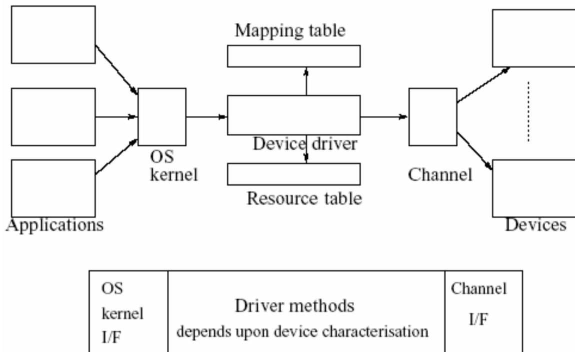
**Figure 5.9: Device-driver interface.**
