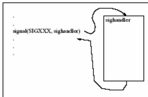
Figure 7.3: Processing signals.
