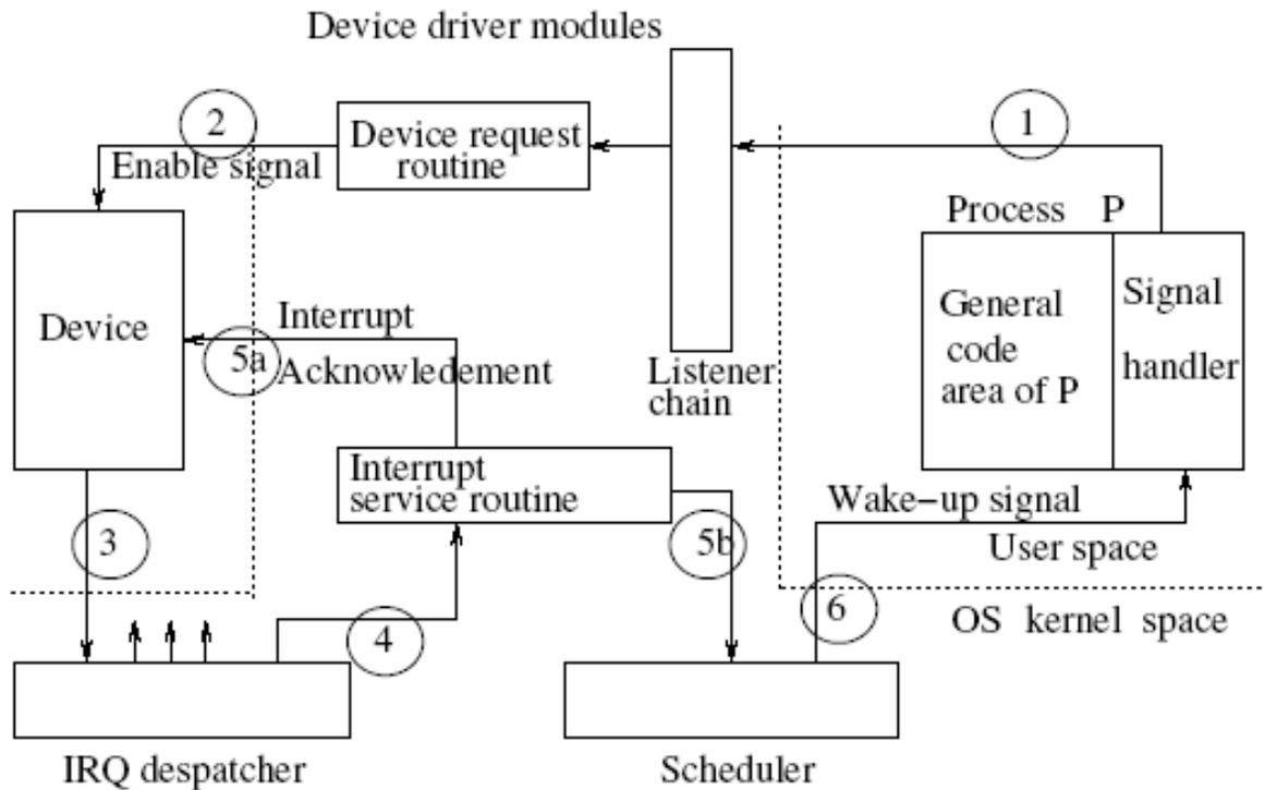
**Figure 5.10: Device-driver operation.**
