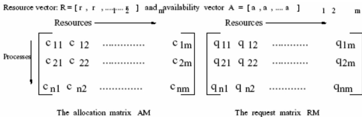
Figure 6.4: Matrix model of requests and allocation.
