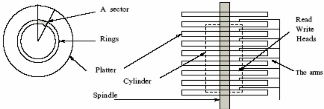
Note that the rings on the disk platters on the spindle form a cylinder. Since all heads are on a particular ring at the same time, so it is easy to organise information on a cylinder. The information is stored in the sectors that can be identified on the rings. sectors are separated from each other. All sectors can hold equal amount of information.
