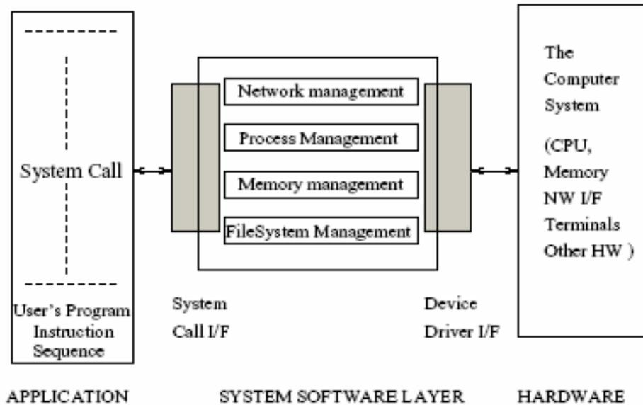
Figure 7.1: Processing system calls.
