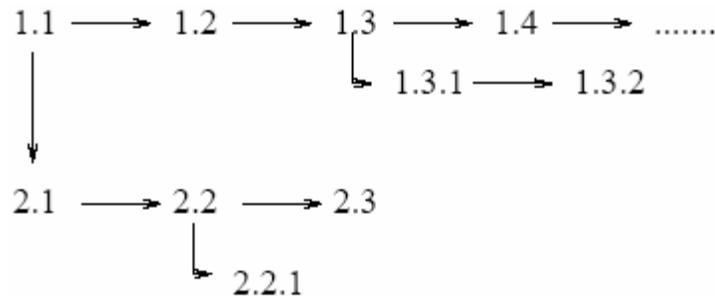
**Figure 17.1: A typical version tree under SCCS.**
