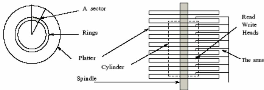
Note that the rings on the disk platters on the spindle form a cylinder. Since all heads are on a particular ring at the same time, so it is easy to organise information on a cylinder. The information is stored in the sectors that can be identified on the rings. sectors are seperated from each other. All sectors can hold equal amount of information.
