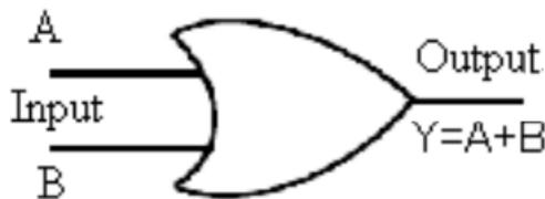
**Figure 3: Graphical symbol for OR gate**
