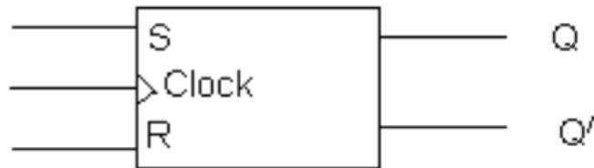
Figure 27: Graphic symbol of RS flip-flop
