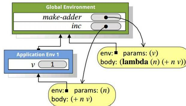
Figure 9.3. Environment after evaluating (define inc (make-adder 1)).
