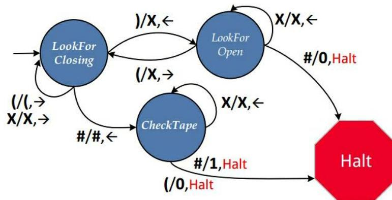
**Figure 6.6. Checking parentheses Turing Machine.**
