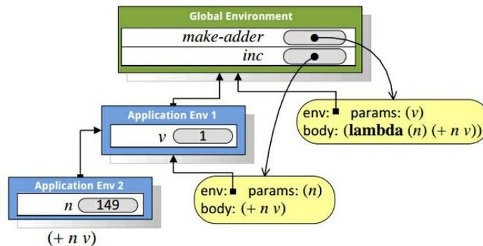
Figure 9.4. Environment for evaluating the body of `(inc 149)`.
