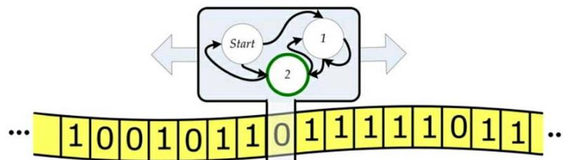
Figure 6.4. Turing Machine model.
