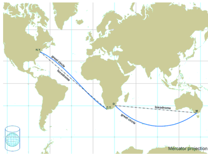
Fig. 3.12: Mercator projection is a cylindrical map projection with a conformal property. The loxodromes in black are straight lines. The great circle lines (orthodromes) in blue are curved.
