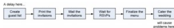
Figure 11.1: An example of problems that can be caused within the critical path.
