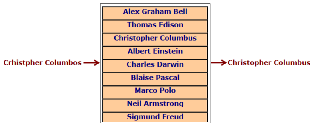
Fig. A content-addressable memory, Input and Output clues with the full name. Similarly, in associative memory, the system can retrieve complete information based on partial input.
