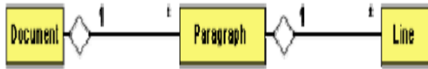
Fig. 7.10: Representation of aggregation
