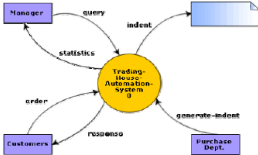
Fig. 5.8: Context diagram for TAS
