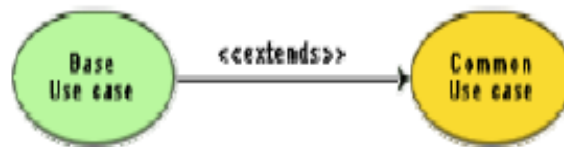
Fig. 7.7: Example use case extension
