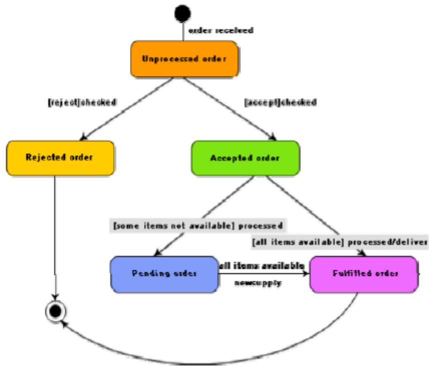
Fig. 7.16: State chart diagram for an order object
