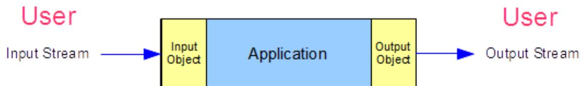
The standard input and output objects of the *iostream* library represent the standard peripheral devices, such as the keyboard and display.
