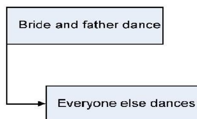
Figure 10.6: A lag means making sure that one task waits a while before it gets started.
