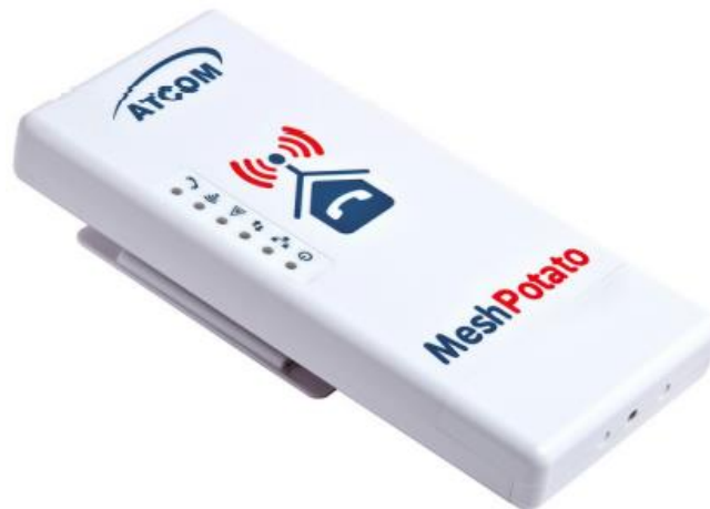
Figure 8.3: Mesh-Potato outdoor mesh WiFi router with VoIP (with one FXS port to connect analog telephone handsets). www.villagetelco.org
