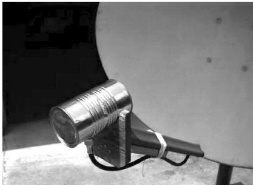
Figure 5.13: Feed horn made from a food can.
