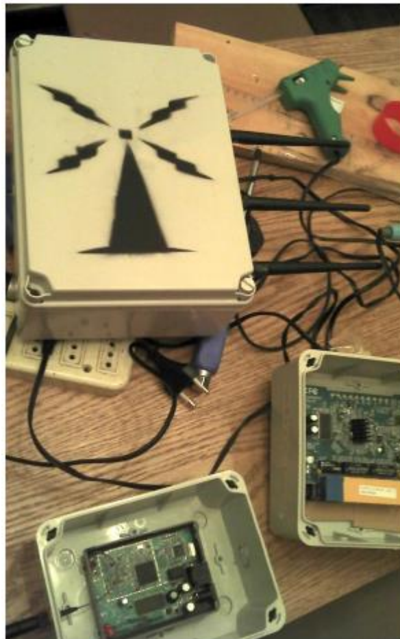
Figure 8.4:DIY outdoor routers based on PCBs taken from SOHO routers (Picture showing two devices based on TP-Link WR741 and WR941 and one based on a Fonera router)
