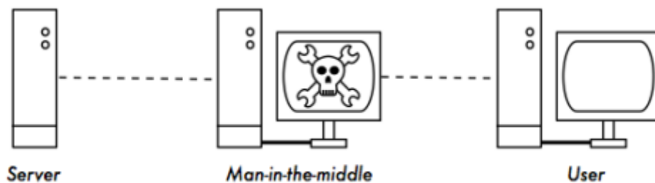
Figure 9.7: The man-in-the-middle effectively controls everything the user sees, and can record and manipulate all traffic. Without a public key infrastructure to verify the authenticity of keys, strong encryption alone cannot protect against this kind of attack.
