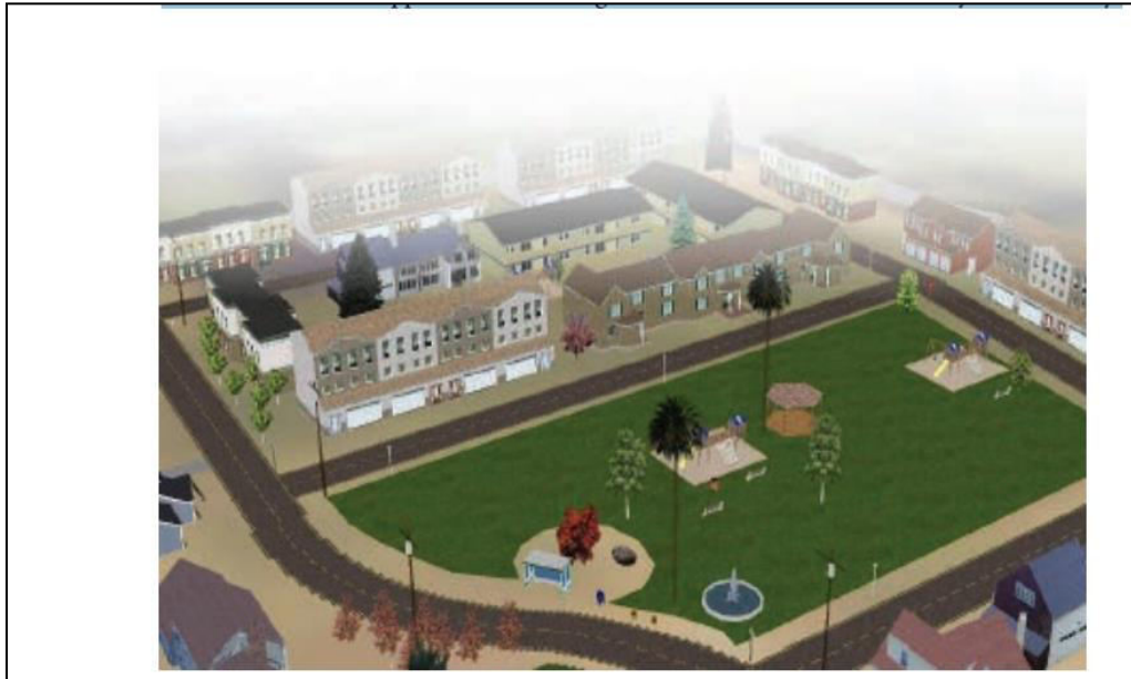
Figure 6.8 A perspective view for a community development scenario. This image was derived from actual data of roads, buildings, and an available parcel in ArcGIS. A proposed community park was incorporated into the plan and visualized using the CommunityViz extension to ArcGIS [12] .
