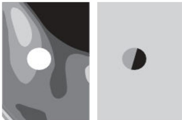
**Figure 5.2:** A circle, in white, is used to retrieve values of cell from raster that is inputted. The output raster covers the same area as the input raster, but there lies no data, which is outside of that particular circular area.
