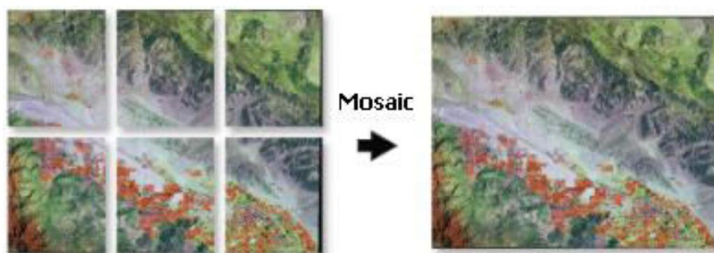
Figure 5.8: The figure illustrates how six neighbouring datasets of raster are mosaicked into a single dataset of raster.
