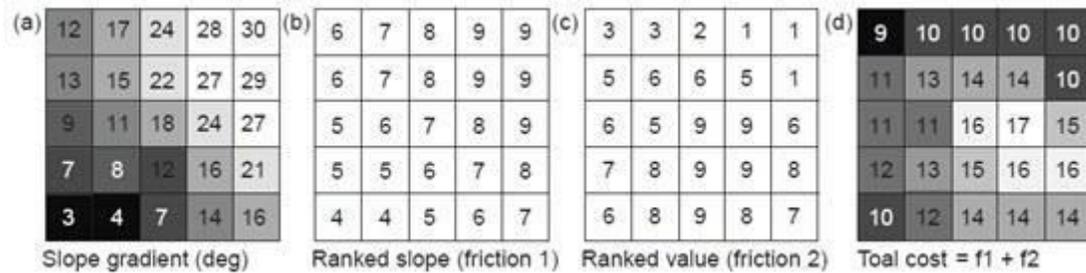
Fig. 7.5 (a) Slope gradient in degrees; (b) ranked (reclassified) slope gradient constituting the first cost or friction input; (c) ranked land value (produced from a separate input land-use raster) representing the second cost or friction input; and (d) total cost raster produced by aggregation of the input friction rasters ( $f_1$  and  $f_2$ ). This total cost raster could then be used within a cost-weighted distance analysis exercise.(Source: Liu and Mason, 2009)
