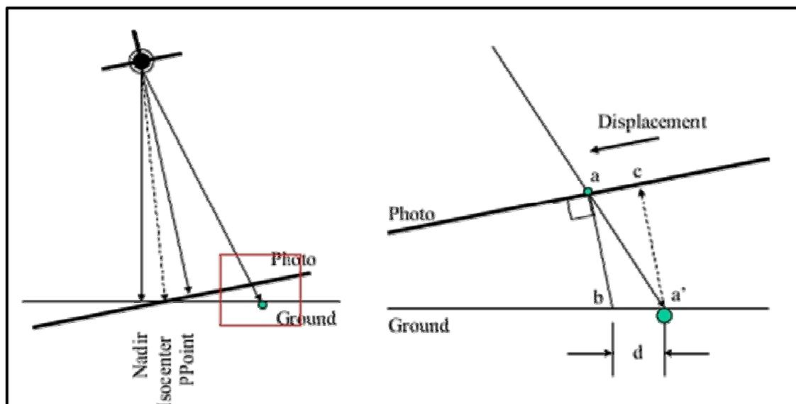
Fig.6.2 Tilt distortion
