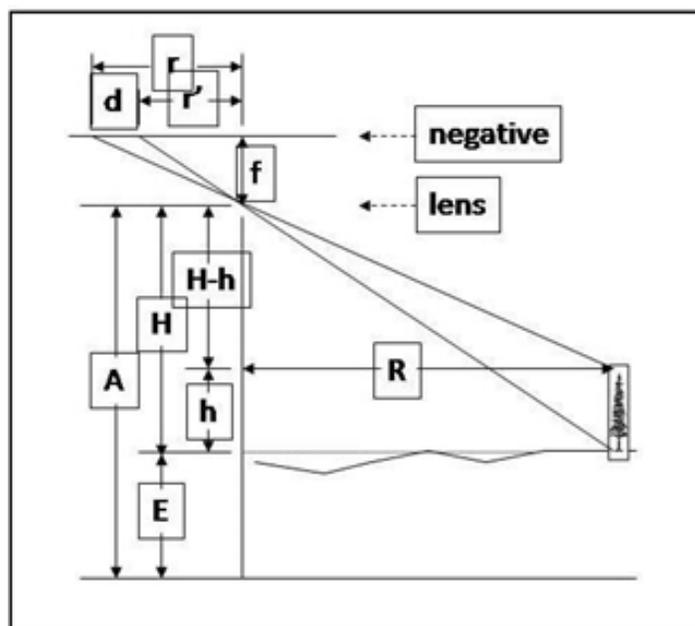
Fig.7.13 Relief Displacement
