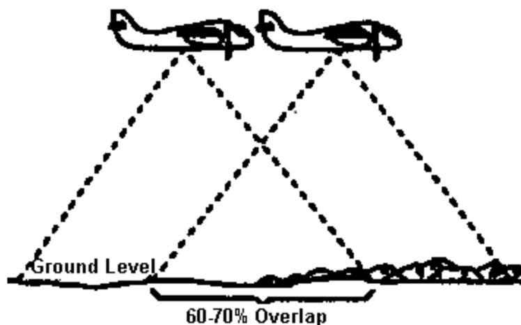
Fig 4.6(a) Overlap required to get the full coverage of area
