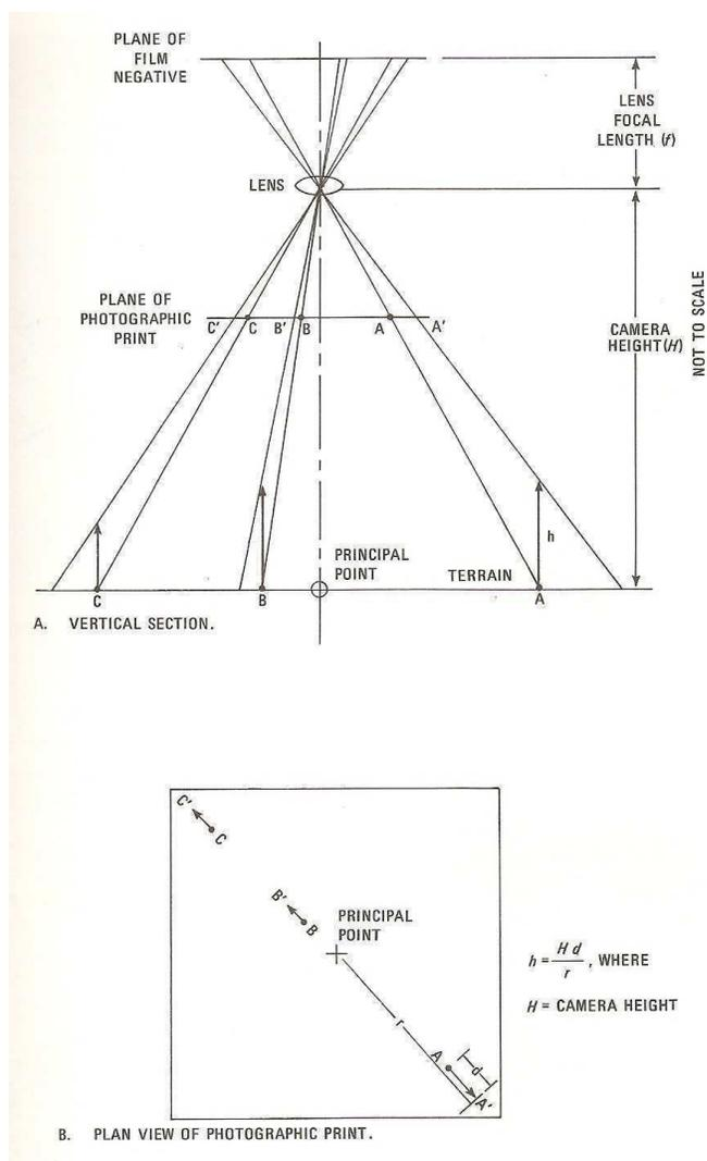
Fig.6.5 Geometry of relief displacement on a vertical aerial photograph
