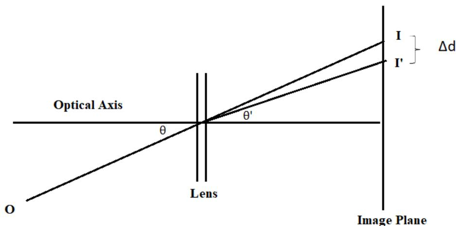
Fig. 6.1 Lens distortion
