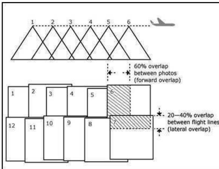
Fig.7.10 Forward and lateral overlapping
