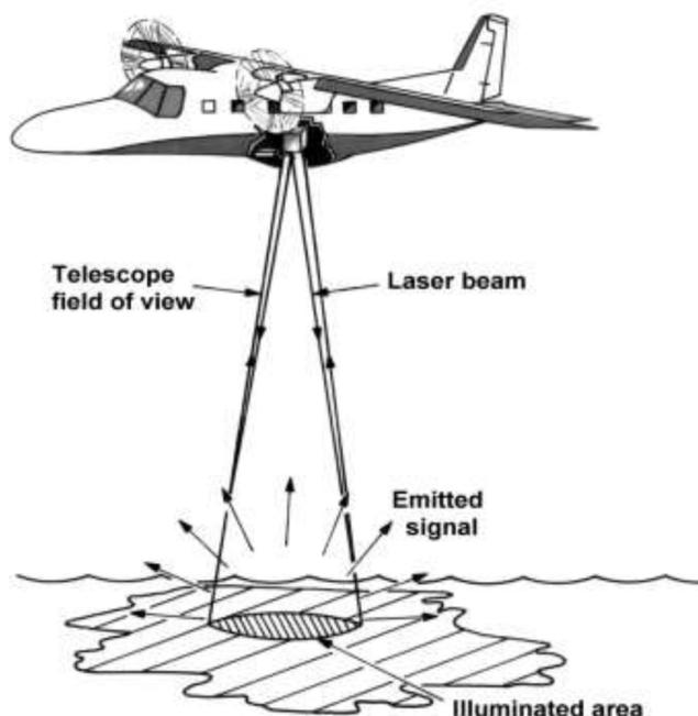
Fig 4.5. Flight direction and signal receiving process
