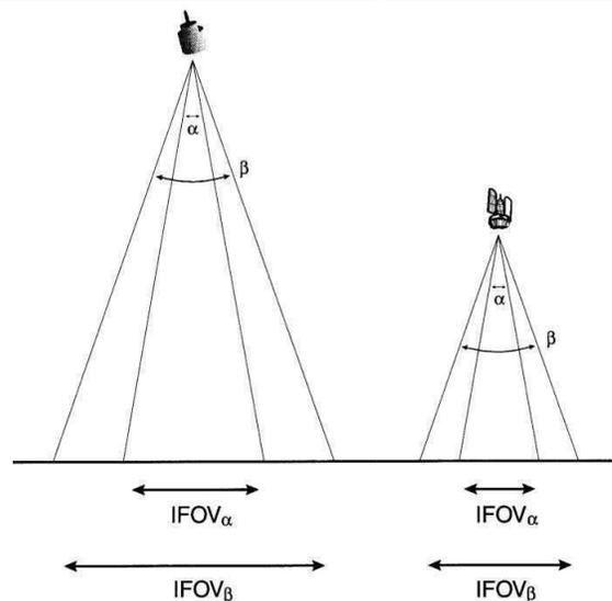
The size of the area viewed on the ground can be obtained by multiplying the IFOV (in radians) by the distance from the ground to the sensor. This area on the ground is called the ground resolution or ground resolution cell. It is also referred as the spatial resolution of the remote sensing system.
