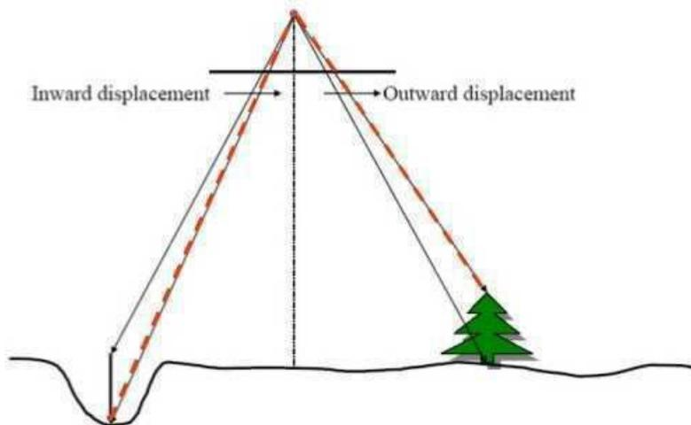
Fig.6.18 Inward and Outward displacement
