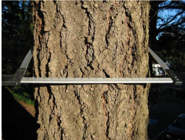
Fig. 1: DBH measurement with caliper
