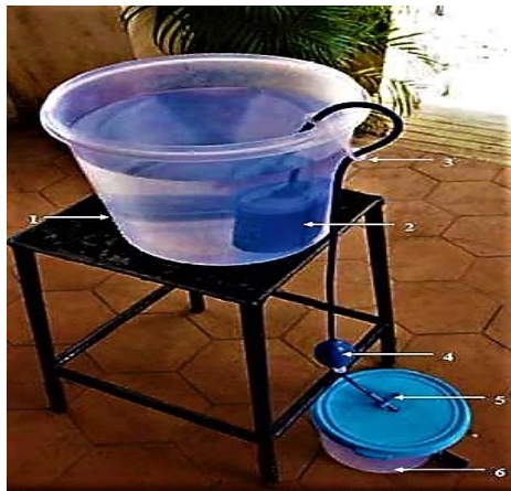
Figure 08: Showing 1. Upper container with contaminated water 2. Plastic jar with filter element and washable pre-filter 3. Plastic connector 4. Rubber bulb to start the filtering process and to clean the element; 5. Opening and closing tap 6. Lower container with lid and tap for storage of drinking water.
