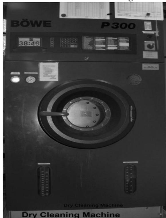
and then fed back into the 'cage'. This is known as the cycle and is continued for the wash duration. The solvent is then removed and sent to a distillation
