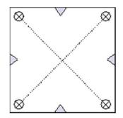
Fig.7.6 Location of the fiducial marks and principal point for an aerial photo image. The intersection of the dotted line indicates the principle point. https://vision-cdc.csiro.au/changs/fiducial/node1.html#fgshapes
