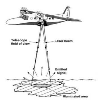
Fig 4.5. Flight direction and signal receiving process Source-http://www.seos-project.eu/modules/laser-rs/laser-rs/c07-p01.html
