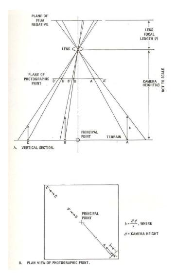
Fig.6.5 Geometry of relief displacement on a vertical aerial photograph
