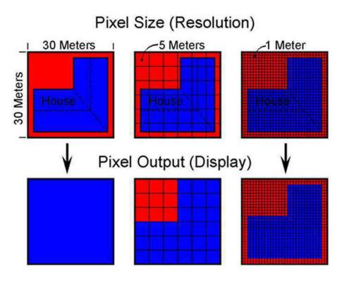
Figure 8.4 Schematic representation of feature identification at different spatial resolutions
