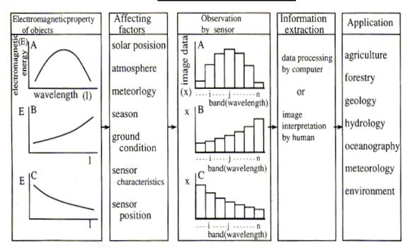
Figure 3. 2 Flow of remote sensing
