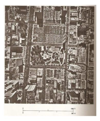
Fig.6.3: Vertical aerial photograph of Long Beach, California, showing relief displacement. Courtesy J. Van Eden.
