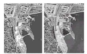
Figure 8.9 Comparison of coarse resolution 2 bit image with a fine resolution 8 bit image
