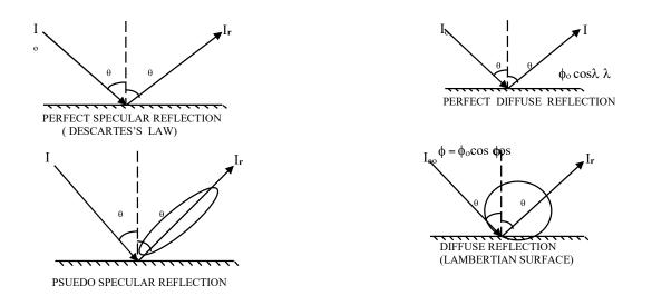
Normally, the reflection is considered the "surface property" of the matter but thorough analysis has revealed that the radiation always "penetrates" the matter and the EMR interaction with the material media takes place in a layer. The thickness of which mainly depends on:
