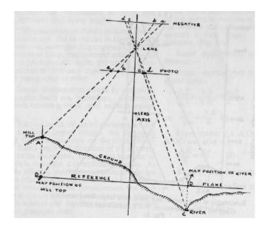
Fig. 6.4: Geometry of displacement due to topographic relief
