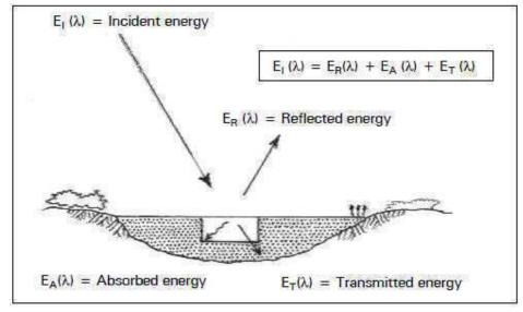
Figure 2.10 Interaction of Energy with the earth's surface
