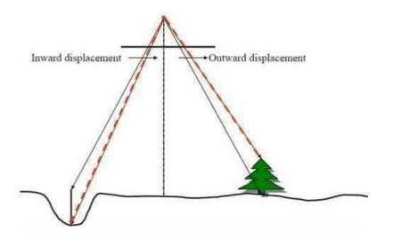
Fig.6.18 Inward and Outward displacement (http://www.edc.uri.edu/nrs/classes/nrs409509/RS/Papers/ReliefDisplacement.pdf)
