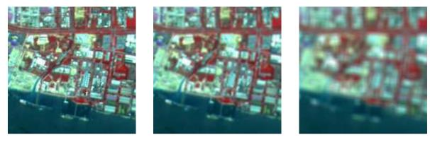
Figure 8.5 An illustration of different spatial resolution for same pixel size
