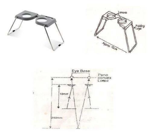
Fig.5.3pocket or Lens stereoscope (Source: Girard, 2003)
