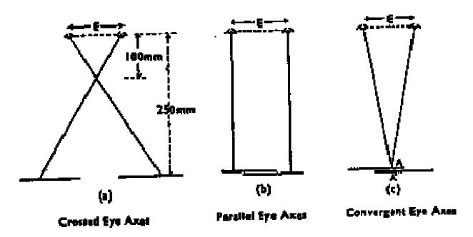
Fig.5.7Three ways of looking at stereoscopic photographs
