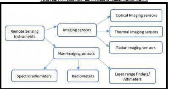
Figure 3.3 Flow chart showing spaceborne remote sensing sensors
