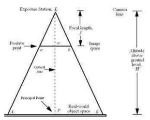
Fig.7.12 Relationship Between the Focal Length (f) and the Aircraft's Flying Height (H):
