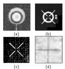
Fig.-7.7Several typical shapes of fiducial mark in an aerial photo image. https://vision-cdc.csiro.au/changs/fiducial/node1.html#fgshapes
