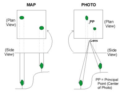
(a) Map (orthographic projection) (b) Photo (perspective projection) varied scale relief displacement
