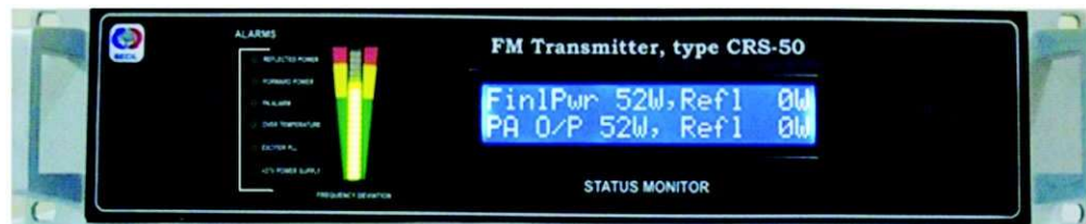
Figure 27.5: Shows the front panel view of BECIL 50 watt FM transmitter type CRS-50
