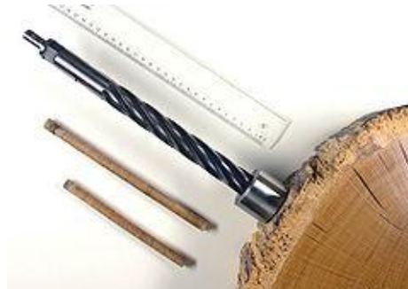
Fig. 12.10. Drill for dendrochronology sampling and growth ring counting
