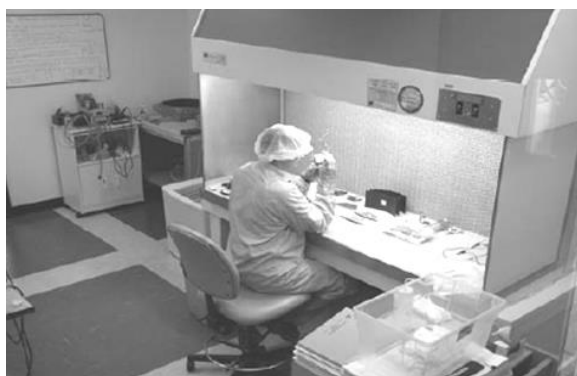
Fig.12.3 Laminar flow (Tissue culture work in sterilized conditions)
