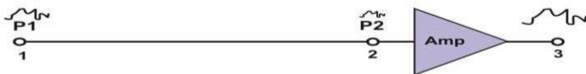
Figure 2.9 Compensation of attenuation using an amplifier
