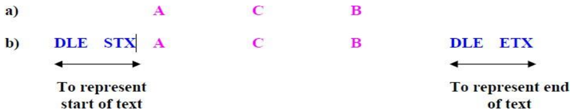
Figure 3.12 Character Oriented (a) Data to be send to the peer, (b) Data after being character stuffed
