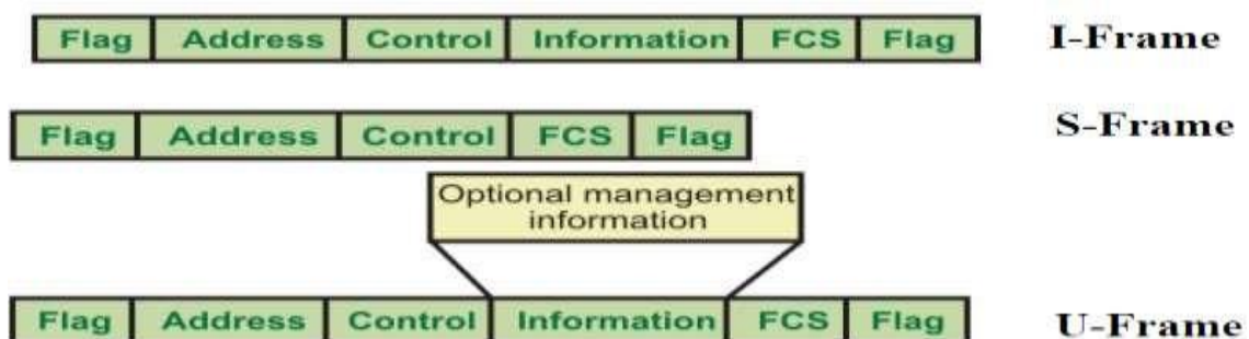
Figure 2.16 Different types of frames used in HDLC
