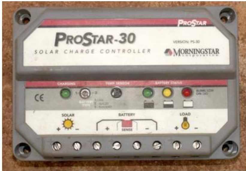
Figure 14.3: A 30 Amp solar charge controller
