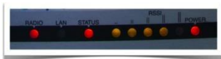
Figure 11.4: The front of a typical Access Point.
