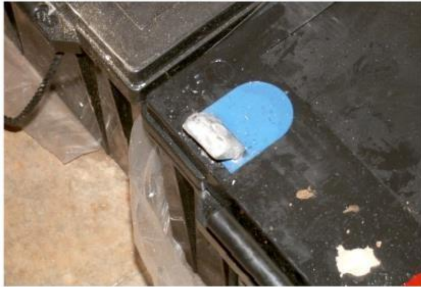
Figure 14.2: A 200 Ah lead-acid battery. The negative terminal was broken due to weight on the terminals during transportation.
