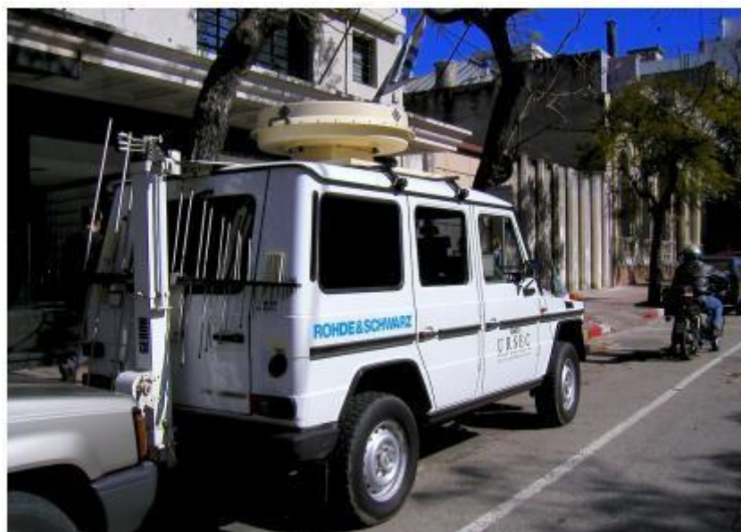
Figure 4.2: A special vehicle for spectrum monitoring in Montevideo, Uruguay.
