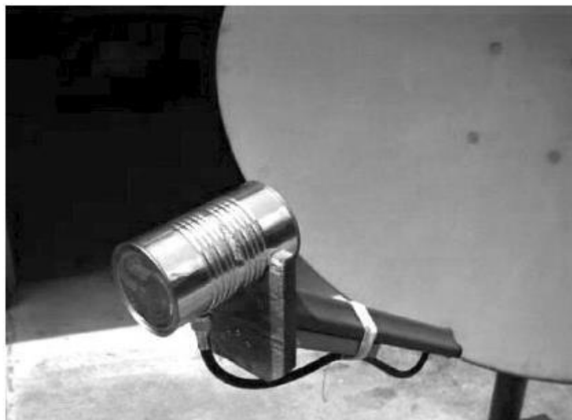
Figure 5.13: Feed horn made from a food can.
