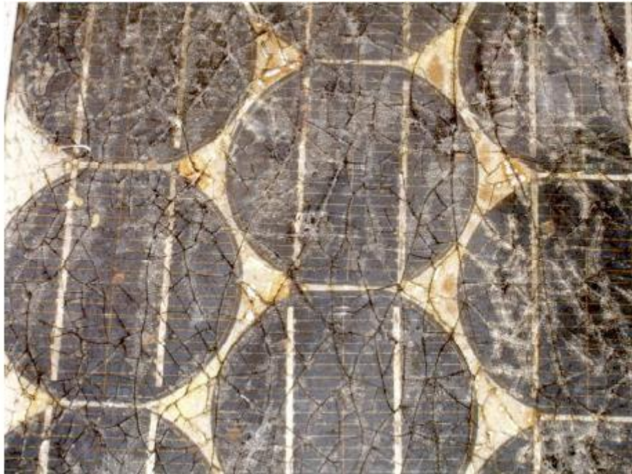
Figure 14.6: The effect of water and corrosion in a solar panel
