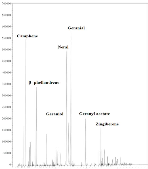
Figure 3: GC chromatogram of oil extracted from blower dried *Z. officinale* rhizomes and geranyl acetate (5.72%). On the other hand, zingiberene (3.10%) and linalool (2.15%) were observed as minor compounds. Thirty-six hours were required to get the constant weight under this drying method (Figure 5; Table 1).
