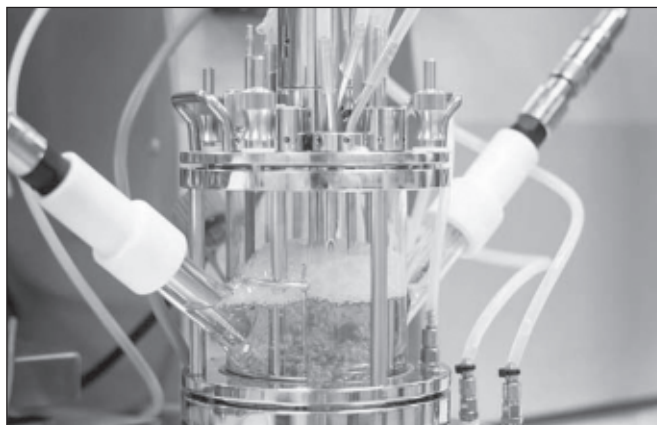
The Carbios process uses an enzyme capable of depolymerizing the PET contained in various plastics or textiles
