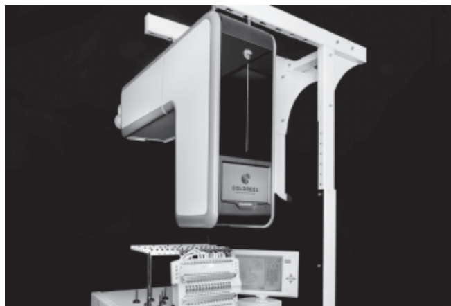
Coloreel's technology enables the high-quality and instant colouring of a textile thread on-demand
