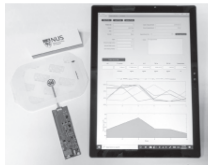
The VeCare platform comprises (clockwise from bottom left) a chip, wound sensor, bandage and app for real-time, point-of-care chronic wound monitoring.
