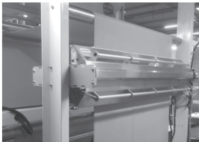
The TexCoat G4 wastes no chemistry during colour, fabric or chemistry changeovers, and only the required chemistry volume is applied to the fabric.
