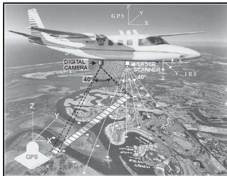
Figure 2.26 Basic Lidar Data Collection Schematic (Jie Shan, Purdue University)
