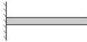
Figure 13: Uniform cylindrical rod fixed at left end.
