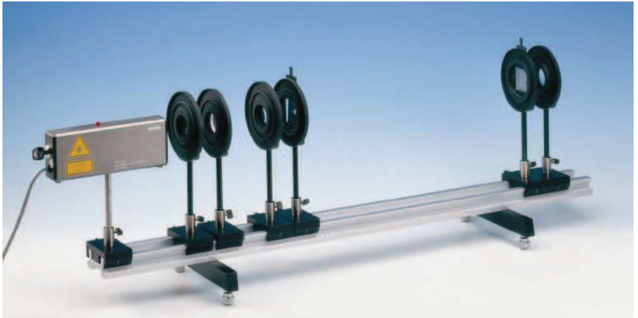
Figure 12: Experimental set-up to determine the different focal lengths of a zone plate
